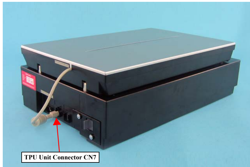
Figure 4-3. Removing the TPU Unit Connector
