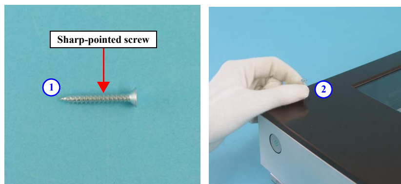
Figure 4-5. Removing the Upper Housing Cap (1)
