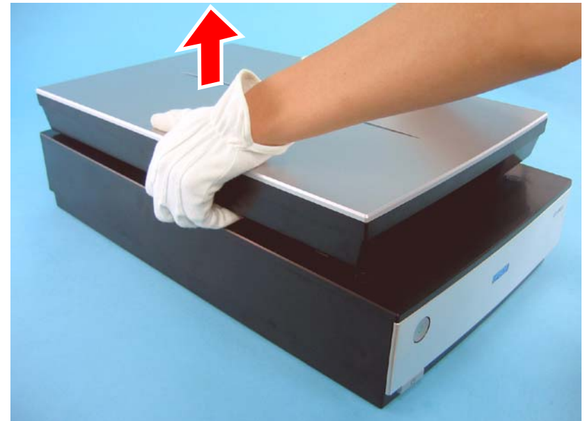
Figure 4-4. Removing the TPU Unit
