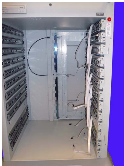
Figure 2-2. Remove the drawers from the AWS
