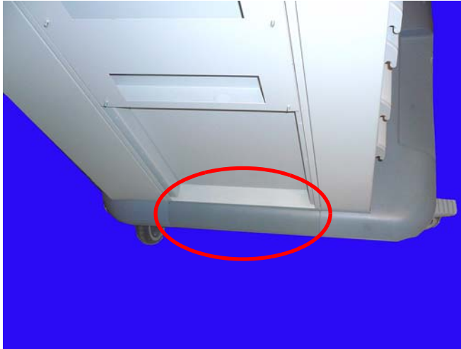
Figure 2-9. Remove the side bumper
