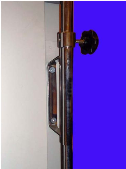
Figure 6-8. Replace the two screws that secure the IV Pole to the AWS
