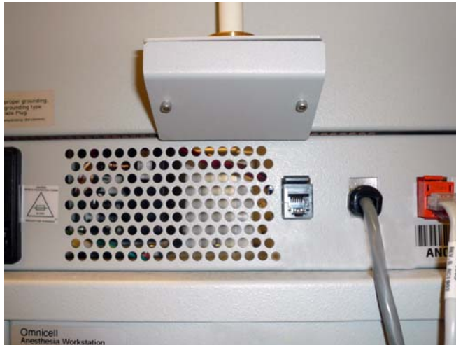
Figure 6-6. Replace the screws that secure the work surface light cover
