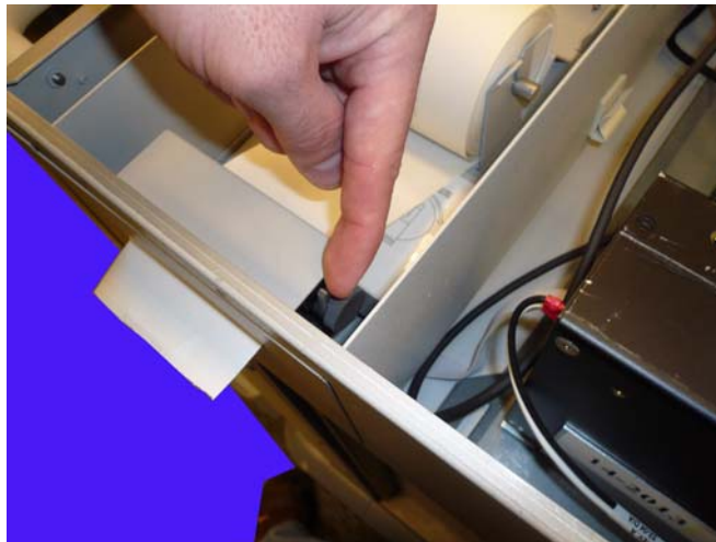
Figure 4-2. Release the printer platen lever
