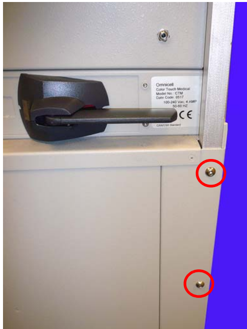
Figure 6-13. Remove the two screws on each side of the AWS
