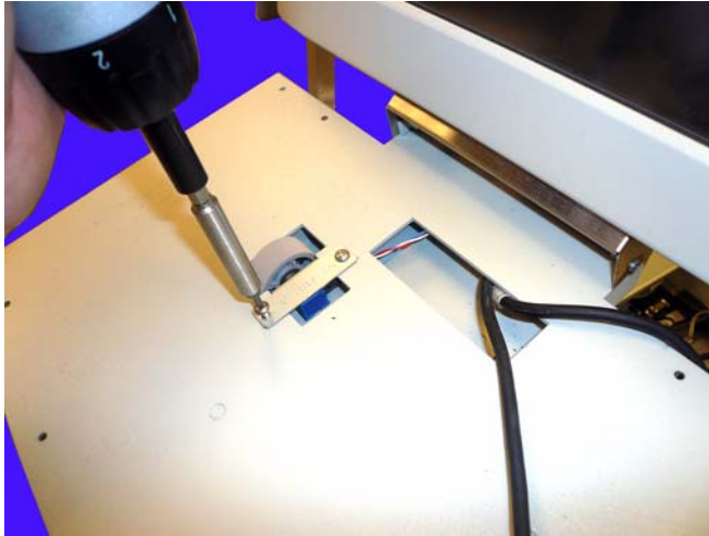
Figure 3-17. Remove the screws securing the potentiometer knob
