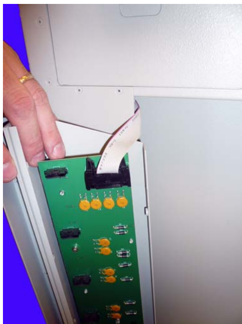
Figure 2-6. Remove the ribbon cable and remove the SPC board from the wireway
