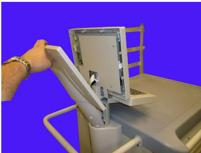
Figure 3-3. Pull back the LCD housing cover
