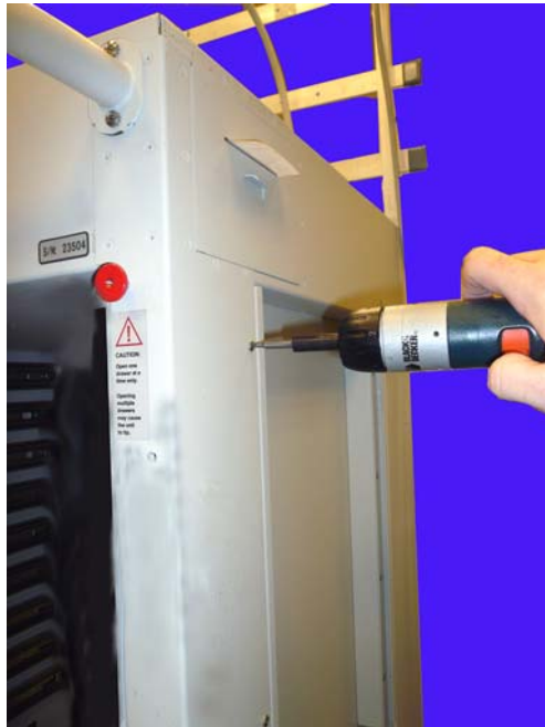
Figure 2-5. Remove the wireway screws on the side of the AWS
