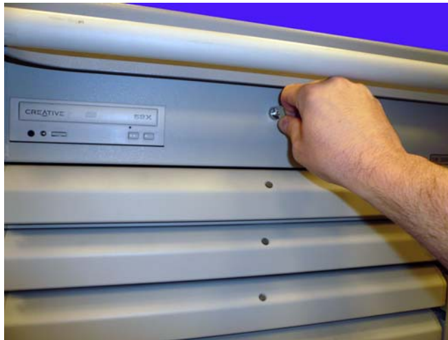
Figure 3-6. Unlock the cam lock that secures the AWS lid
