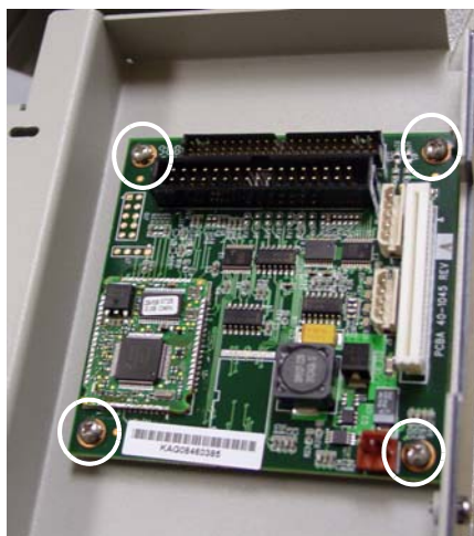
Figure 4-14. Remove the screws that secure the printer control board to the base.
