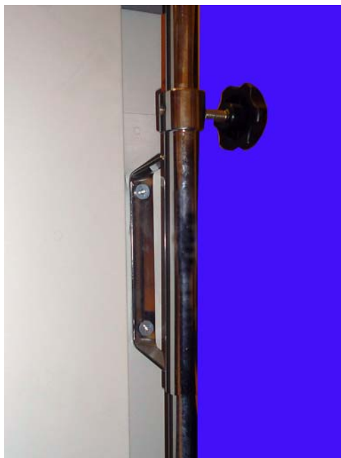
Figure 6-7. Remove the two screws that secure the IV Pole to the AWS
