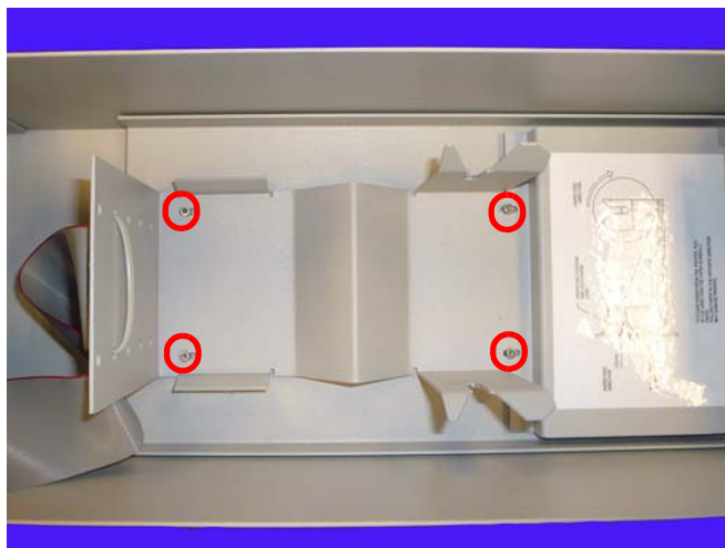
Figure 4-4. Remove the four screws that secure the printer base to the drawer bottom
