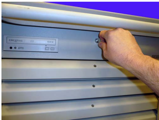
Figure 1-1. Unlock the cam lock that secures the AWS lid
