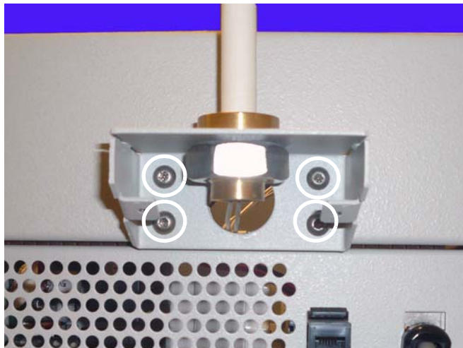
Figure 6-4. Remove the screws that secure the work surface light to the AWS
