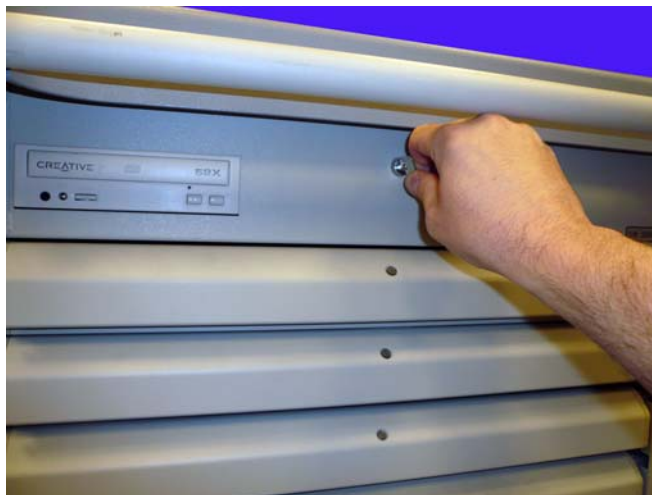
Figure 4-1. Unlock the cam lock that secures the AWS lid
