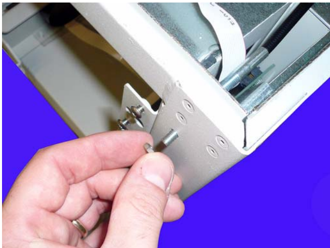
Figure 2-15. Remove the nut that secures the manual override cable to the frame.
