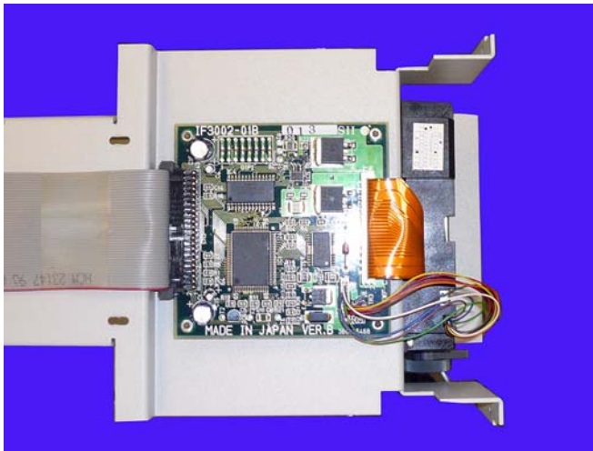
Figure 4-7. Remove the screws that secure the printer control board to the base.
