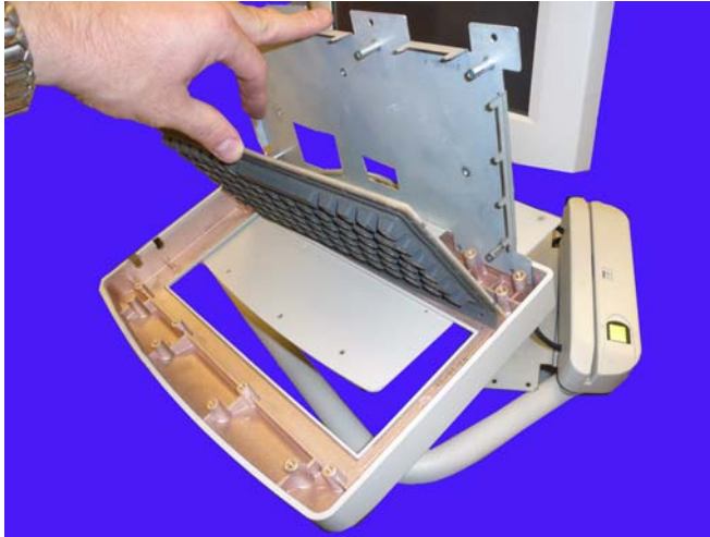
Figure 3-13. Remove the keyboard
