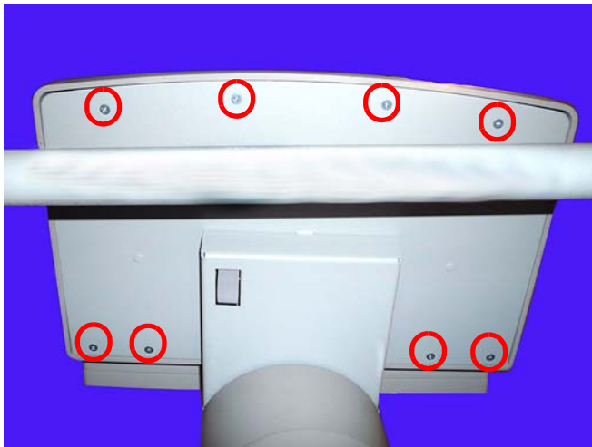
Figure 3-8. Remove the screws securing the keyboard housing
