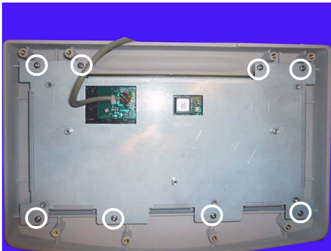
Figure 3-10. Remove the screws that secure the keyboard bezel
