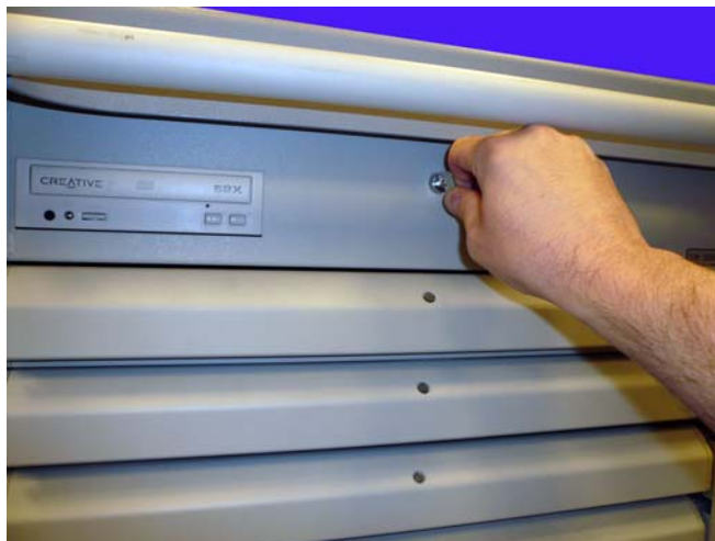
Figure 6-1. Unlock the cam lock that secures the AWS lid
