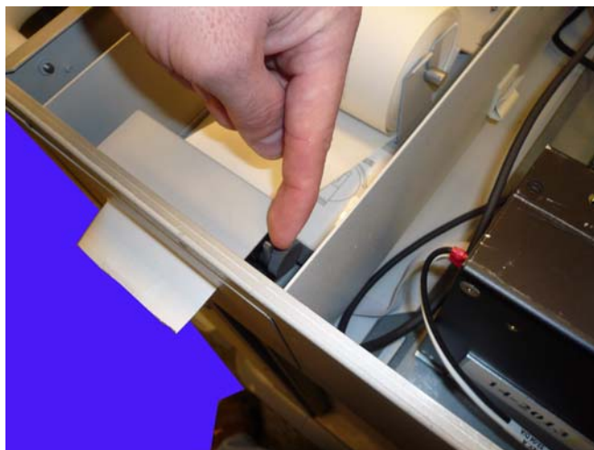
Figure 2-11. Push the platen lever toward the frame to release the paper
