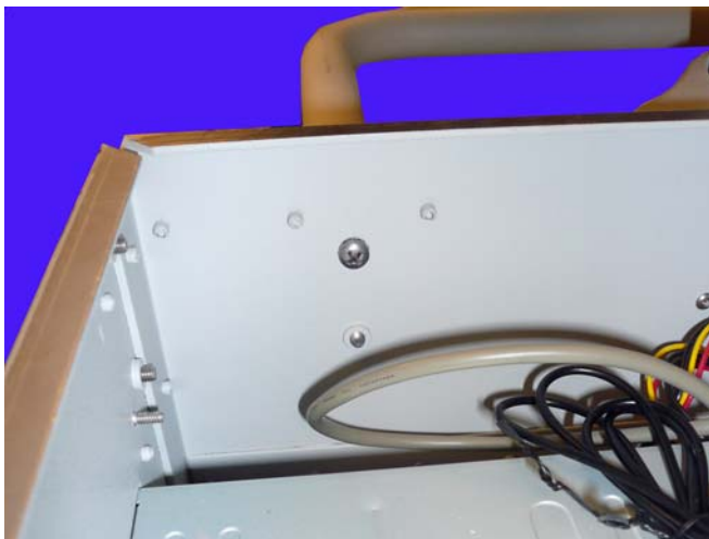
Figure 2-20. Remove the screw that secures the transport handle to the inside of the frame
