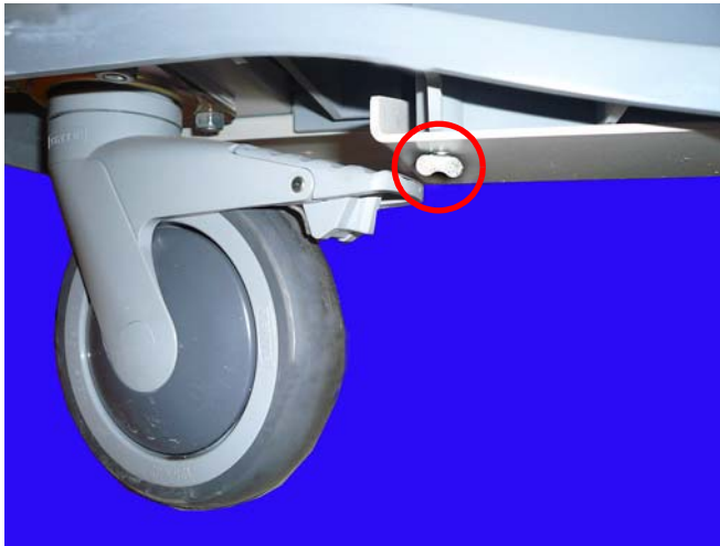
Figure 2-7. AWS Bumper torque screws
