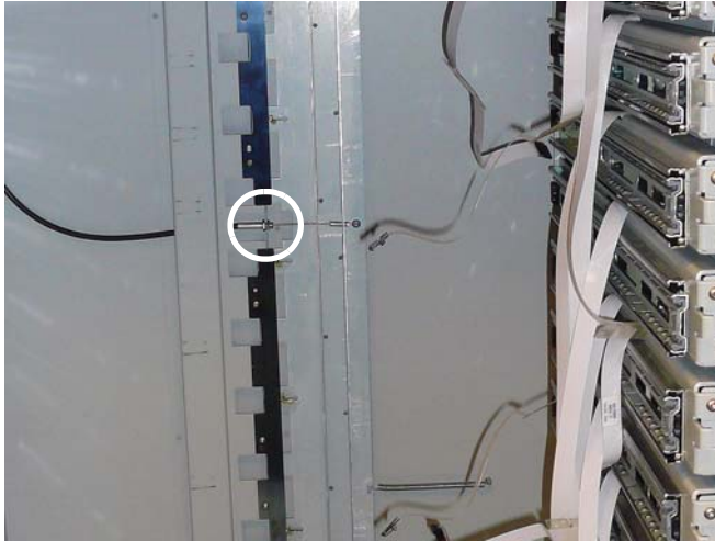
Figure 2-17. Loosen the nut that secures the cable to the frame anchor
