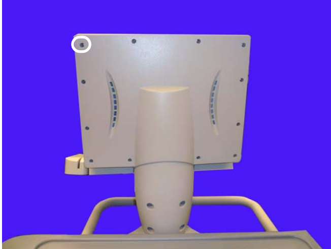
Figure 3-2. Remove the screws securing the housing
