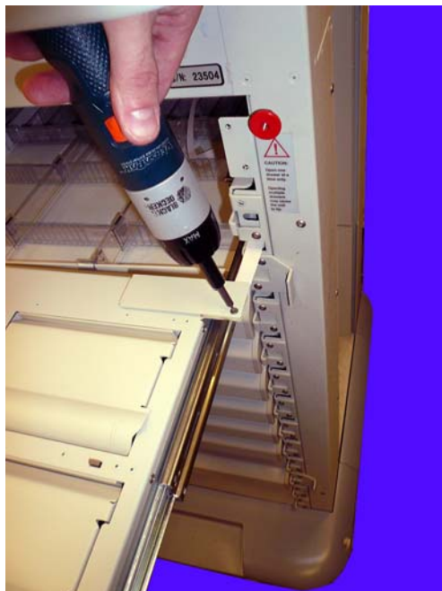
Figure 5-2. Remove the Controller Cable Cover
