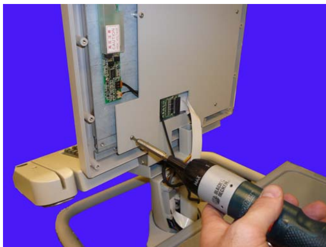
Figure 3-5. Remove the screws securing the metal housing plate
