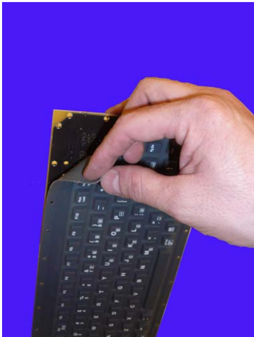
Figure 3-14. Remove the elastomer
