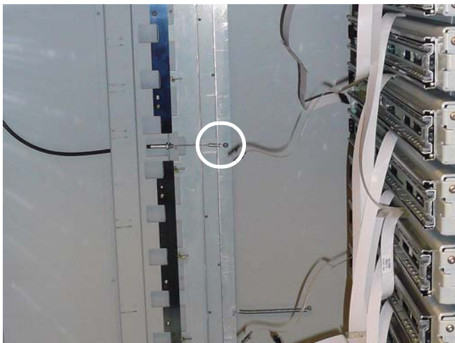
Figure 2-16. Remove the screw that secures the cable to the manual override assembly.
