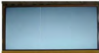
Vertical Line Source TAB IC Defect
