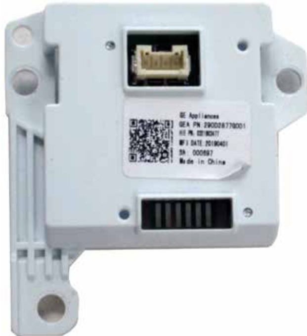
J901 DC Voltage Comm in from Main Board
