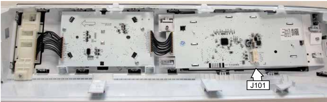
J101 DC Voltage in from Main Board and Communication Out to Main Board
