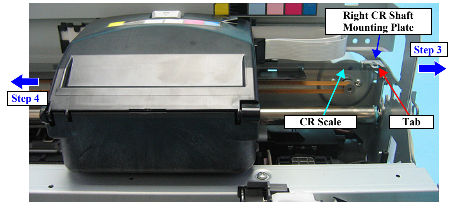
Figure 4-40. Drawing Out the CR Scale
