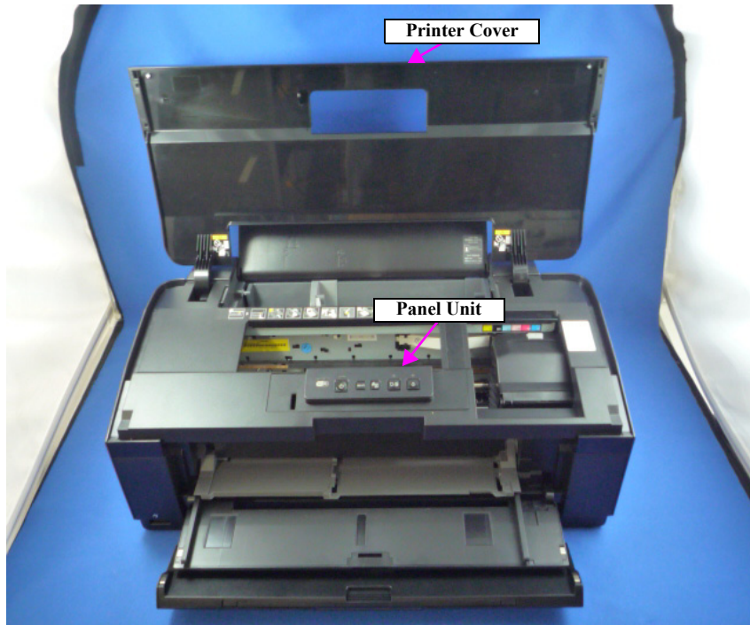
Figure 8-9. Removing the Panel Unit (1)
