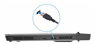
**4** Connect a USB Type-C to Type-A dongle to the Thunderbolt 3 (USB Type-C) port on the back side of your computer.
