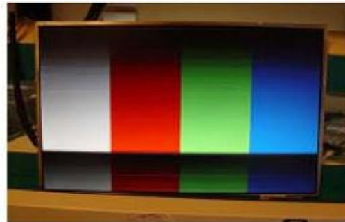
Horizontal Block Gate TAB IC Defect
