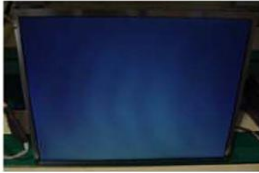
Panel Mura, Light leakage
