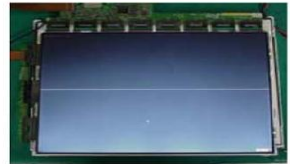
Horizontal line Gate TAB IC Defect
