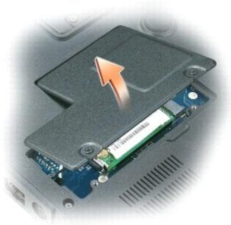
4. If a Mini-Card is not already installed, go to [step 5](#). If you are replacing a Mini-Card, remove the existing card:
