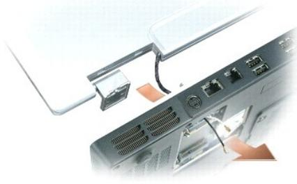
2. Align the display assembly over the screw holes in the base of the computer.
