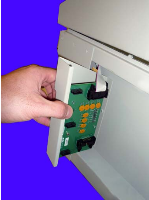
Figure 2-4. Disconnect the ribbon cable and remove the SPC board
