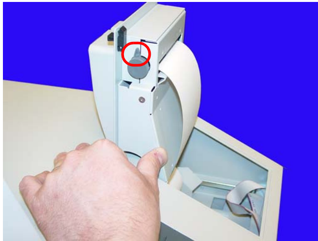
Figure 1-6. Turn the Platen Lever to the Left and Remove the Paper
