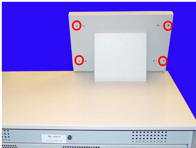
Figure 1-1. Remove the Four Outer Screws
