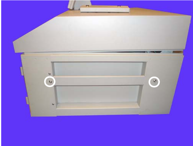
Figure 2-2. Remove the two screws securing the transport handle
