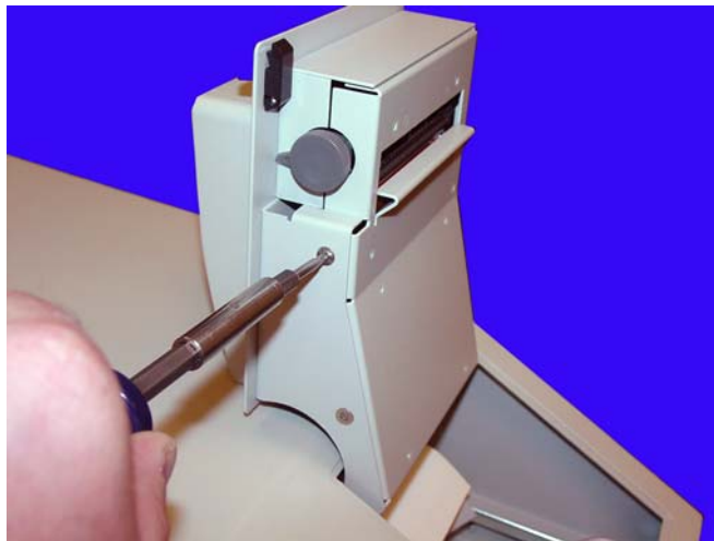
Figure 1-7. Remove the Screws Securing the Printer Assembly
