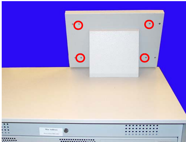
Figure 1-2. Remove the Four Inner Screws
