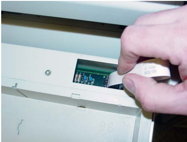
Figure 3-5. Connect the drawer controller cable to the controller board
