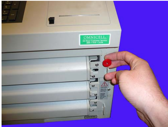
Figure 3-8. Pull the manual override lever
