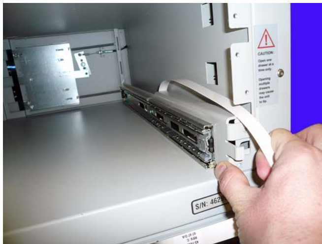
Figure 3-6. Install the new slide support bracket
