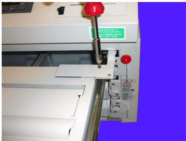
Figure 3-9. Remove the controller cable cover
