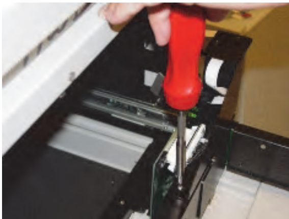
Figure 5-69. Removing the rail cable bracket: 6-32 button-head screw
