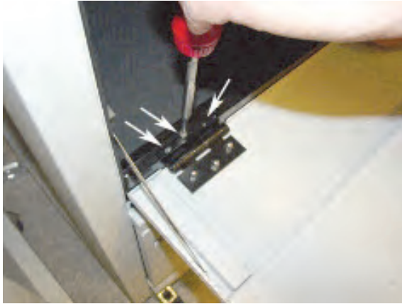
Figure 5-20. Attaching the door hinges
