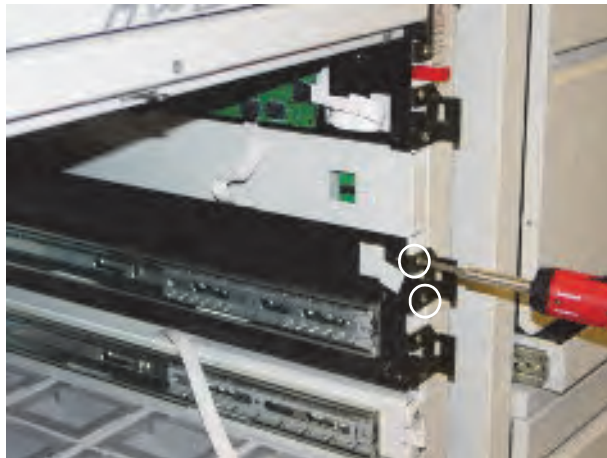
Figure 5-38. Removing the bottom bayonet
