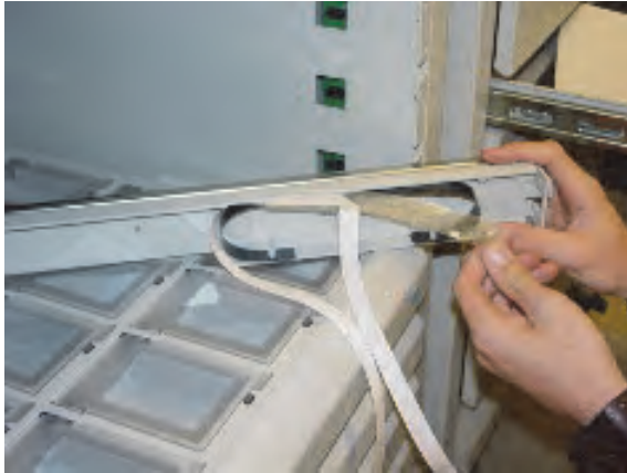
Figure 5-41. Inserting the new dispense drawer cable into the drawer bayonet
