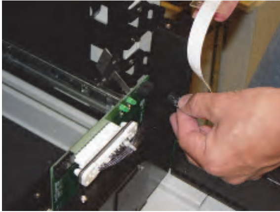
Figure 5-70. Disconnecting the rail cable from the rail controller board
