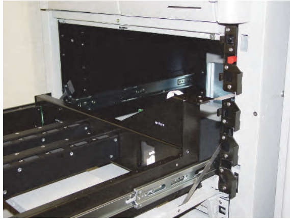
Figure 5-31. Extending the rail frame
