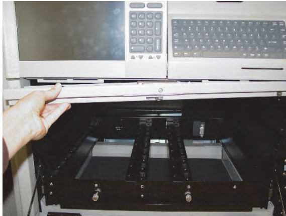
Figure 5-64. Sliding the top crossbar into position
