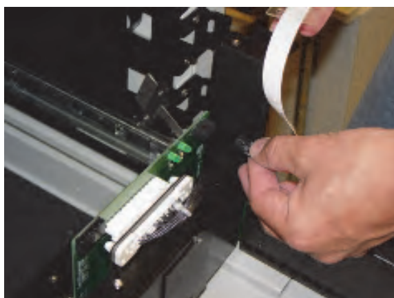
Figure 5-77. Connecting the rail cable from the rail controller board
