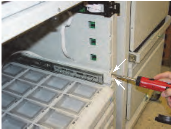
Figure 5-43. Installing the drawer bayonet
