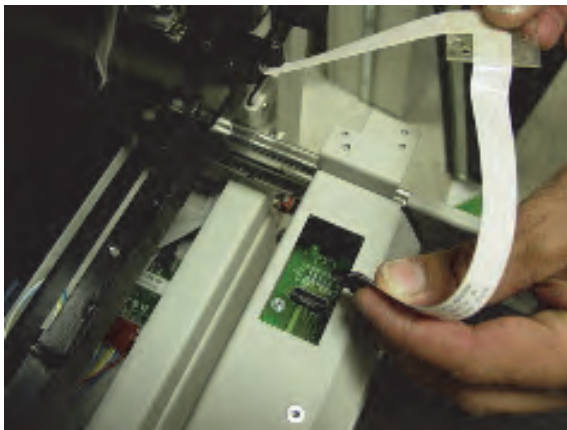
Figure 5-50. Connecting the drawer cable
