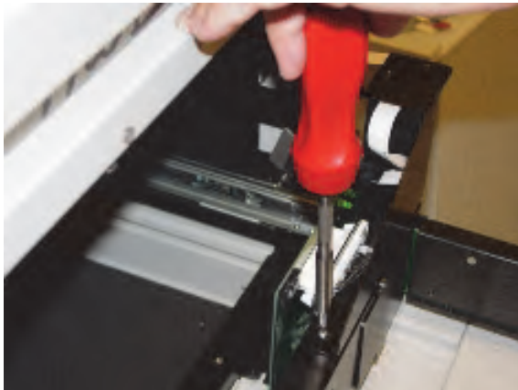
Figure 5-4. Removing the rail cable bracket (6-32 button-head screws)
