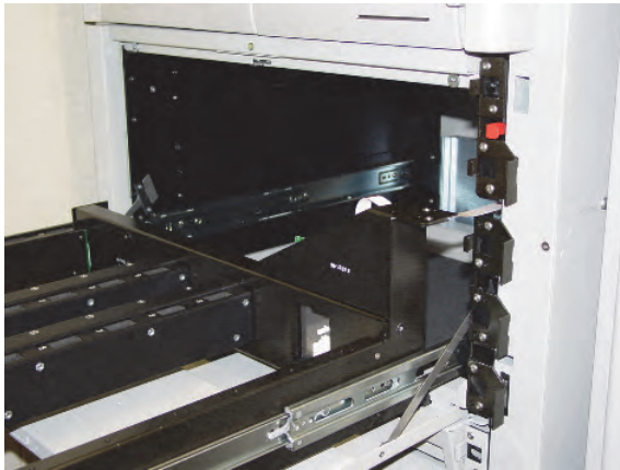
Figure 5-9. Extending the rail frame
