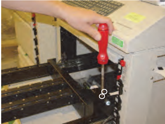
Figure 5-3. Removing the rail cable bracket (6-32 flat-head screws)
