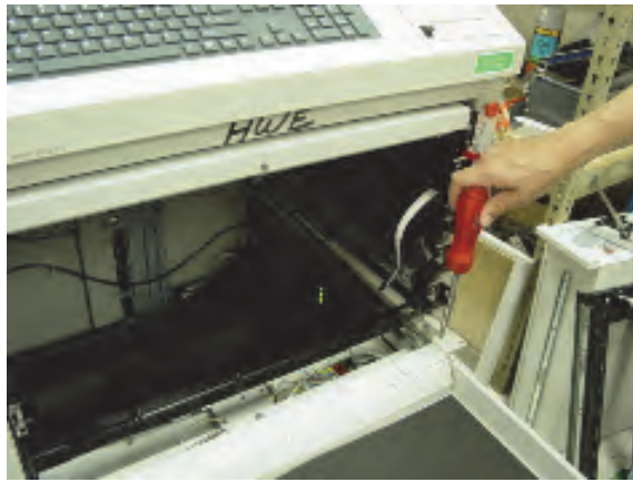
Figure 5-51. Installing the drawer cable bracket
