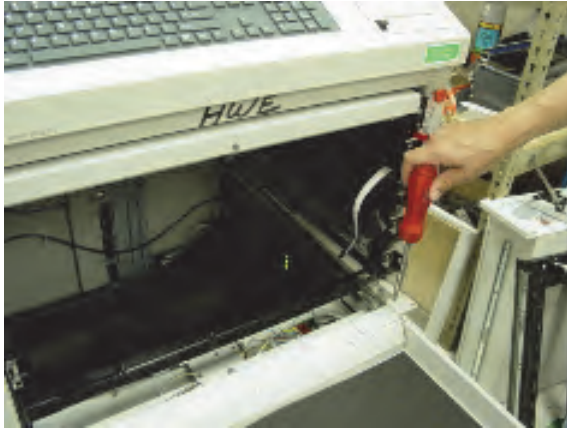
Figure 5-30. Installing the drawer cable bracket
