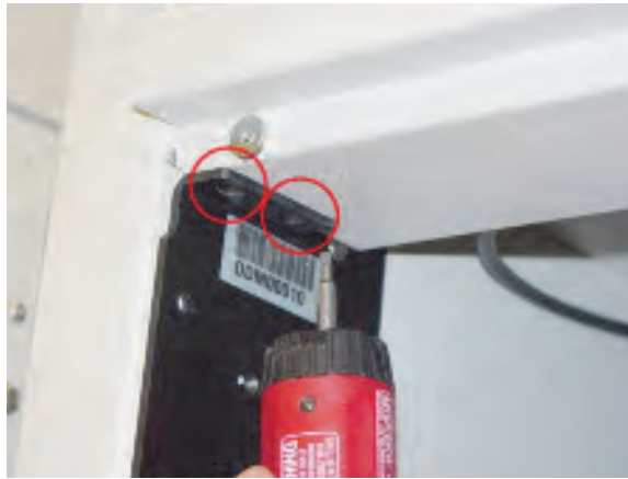
Figure 5-66. Installing the top crossbar: two 8-32 flat-head screws
