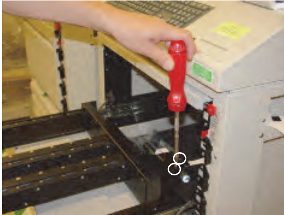
Figure 5-68. Removing the rail cable bracket: two 6-32 flat-head screws
