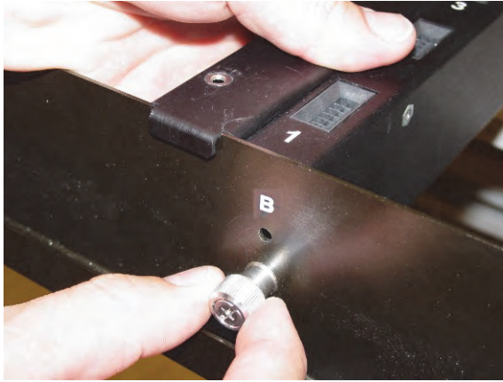
Figure 4-3. Tightening the Mounting Screw
