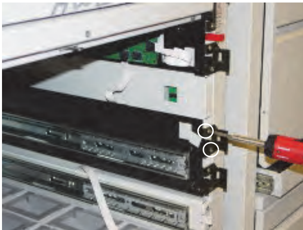
Figure 5-44. Installing the bottom bayonet
