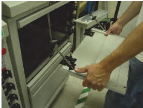
Figure 5-32. Removing the restock door
