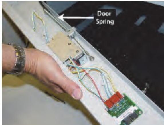
Figure 5-62. Secure the door release cable to the top crossbar
