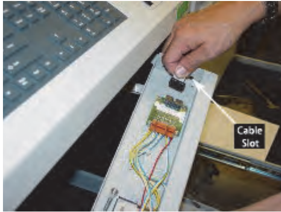
Figure 5-54. Disconnecting the ribbon cable
