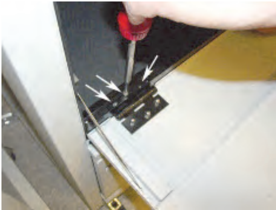
Figure 5-19. Detaching the door hinges
