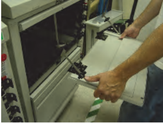
Figure 5-24. Removing the restock door
