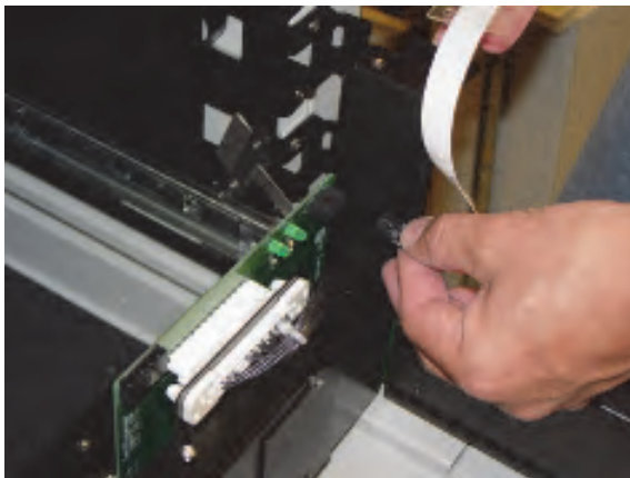
Figure 5-8. Connecting the rail cable
