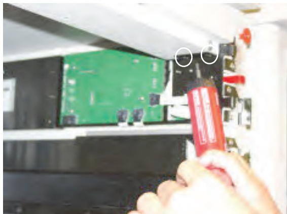
Figure 5-65. Installing the top crossbar: two 8-32 flat-head screws
