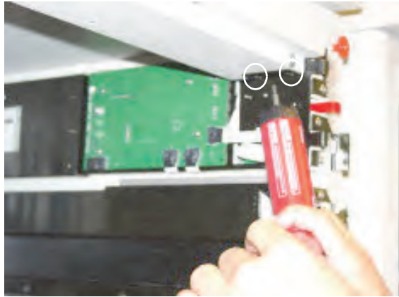
Figure 5-52. Removing the top crossbar: two 8-32 flat-head screws
