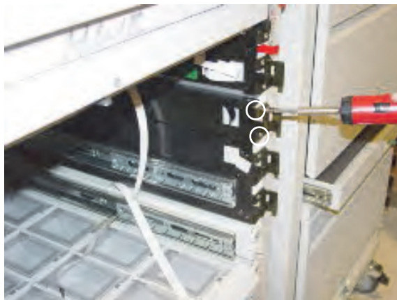
Figure 5-75. Installing the middle bayonet
