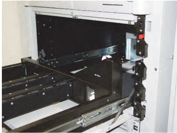
Figure 5-14. Extending the rail frame
