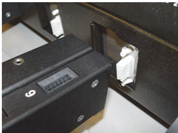
Figure 5-12. Connecting rail back to connector
