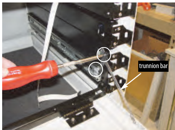
Figure 5-17. Detaching the trunnion bars
