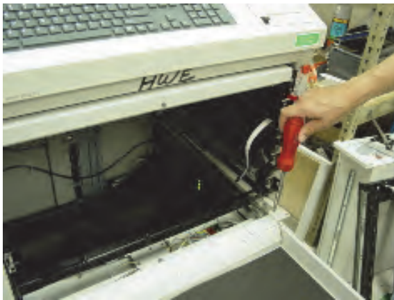
Figure 5-25. Removing the drawer cable bracket
