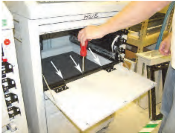
Figure 5-18. Removing the fix inhibitor bracket
