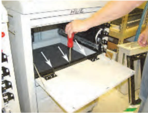
Figure 5-22. Installing the fix inhibitor bracket
