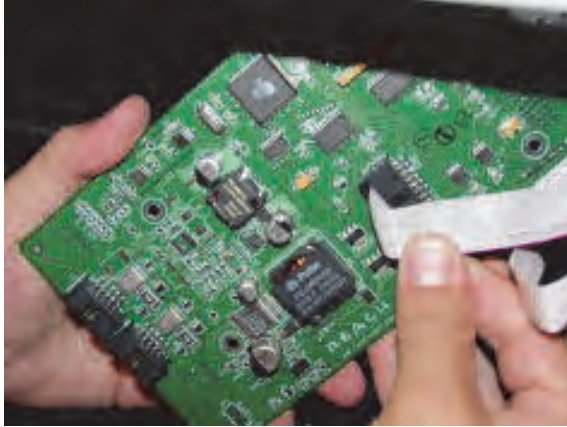
Figure 5-80. Connecting the ribbon cable
