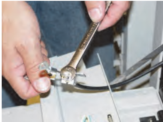
Figure 5-59. Inserting the door release bracket tab between the hex nuts
