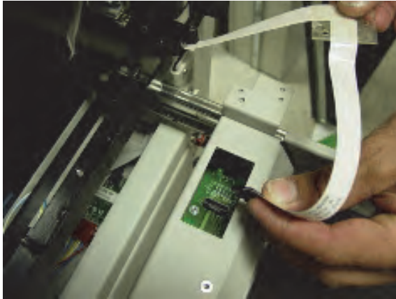
Figure 5-26. Disconnecting the drawer cable
