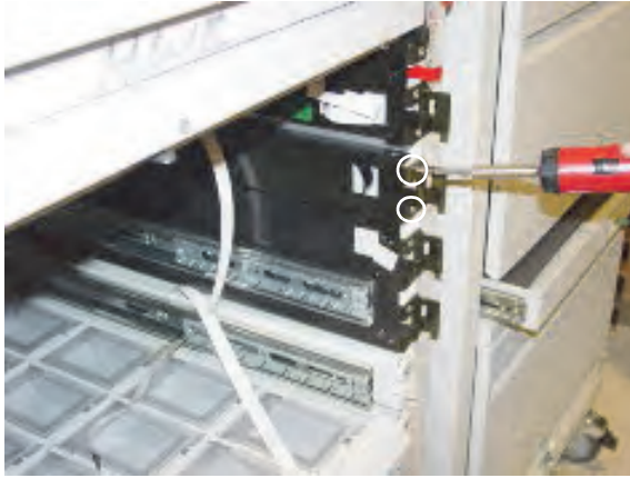
Figure 5-72. Removing the middle bayonet
