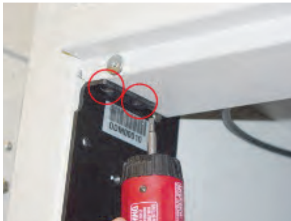
Figure 5-53. Removing the top crossbar: two 8-32 flat-head screws
