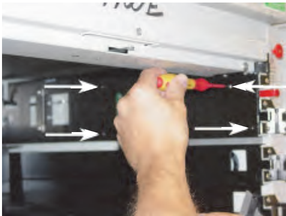
Figure 5-71. Removing the carrier controller cover
