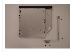
**Step 12.** Position the New ODD (Label side down) The Bracket should be aligned on the Right side of the ODD. Take note of the proper alignment of the screw holes.
