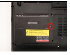
**Step 16.** Reinstall the ODD Bay screw to secure the ODD Assembly.
