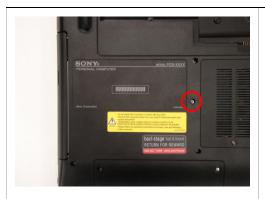
**Step 4.** Using the enclosed magnetic screwdriver, remove the screw securing the ODD Bay. Put aside the ODD Bay screw to re-secure the ODD Bay later in the procedure.
