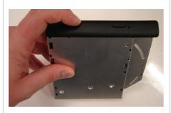
**Step 11.** Align the tabs on the Bezel with the tab holes located on the ODD. Carefully press the Bezel into place.
