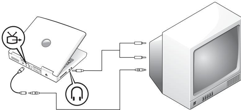
To connect the computer to a television that has a composite video input only, use a composite TV-out adapter cable. Before you begin, ensure that you have the following cables:
