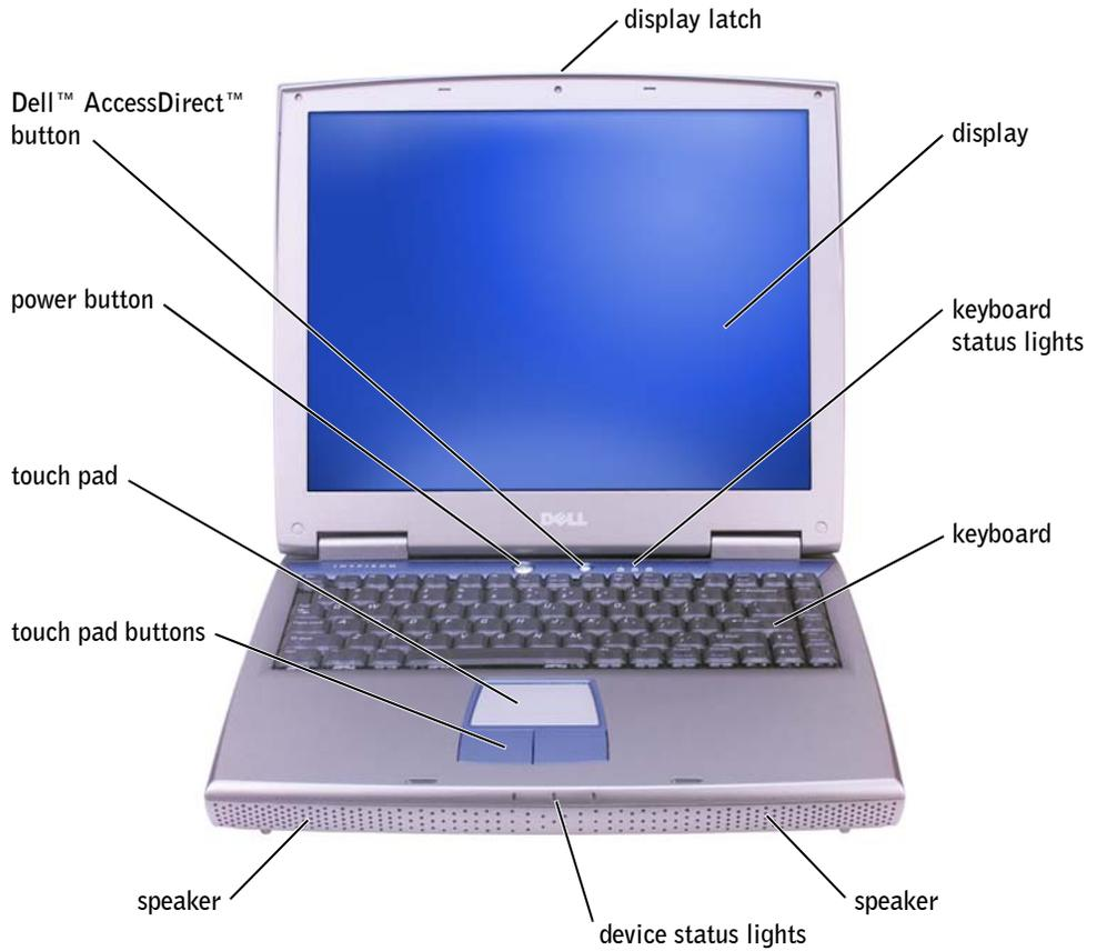
**DISPLAY LATCH** — Keeps the display closed.
