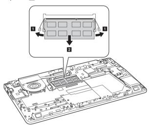
When installing: Insert the notched end of the DIMM into the socket. Push the DIMM firmly, and pivot it until it snaps into the place. Make sure that it is firmly fixed in the slot and difficult to be moved.
