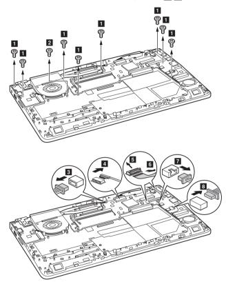
When installing: Make sure that all the connectors are attached firmly.
