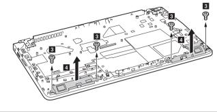
Remove four screws 3, and then remove the speakers in the direction shown by arrows 4.
