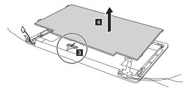
When installing: Make sure that the connector is attached firmly.
