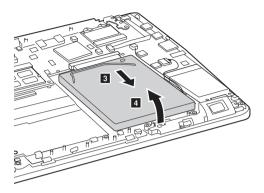
When installing: Make sure that the HDD connector is attached firmly.
