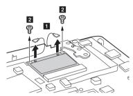
In step **1**, unplug the jacks by using the removal tool antenna RF connector (P/N: 08K7159), or pick up the connectors with your fingers and gently unplug them in the direction shown by arrows.
