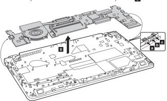
Figure 8. Removal steps of system board (continued) Remove the system board in the direction shown by arrow **[9**].
