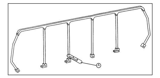
There is a bolt in the folddown siderail latch (A) that holds the siderail in the upright position or in an intermediate position. Lift up on the siderail and be sure the bolt engages and the siderail is securely latched. To lower the siderail, push up on the latch (A) until the bolt disengages and guide the siderail down.
