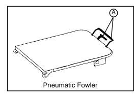
To position the pneumatic Fowler, grasp the handles (A) and squeeze. Guide the Fowler to the desired height and release the handles.
