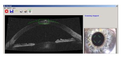
SL-OCT can image in any cross-section from horizontal to vertical. The slit beam (on the patient's eye and/or in the video image) shows the location of the OCT scan.
