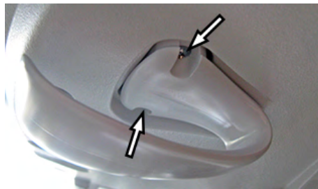
Figure 8-26 loosen 2 screws and remove cable holder
