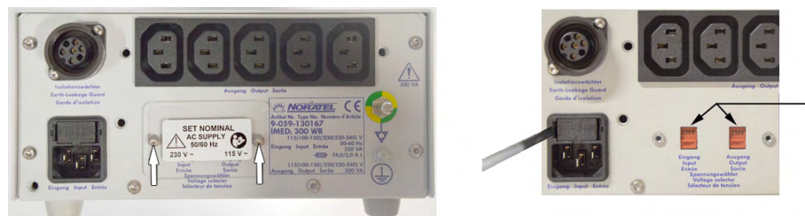
Figure 8-35 change input/output voltage
