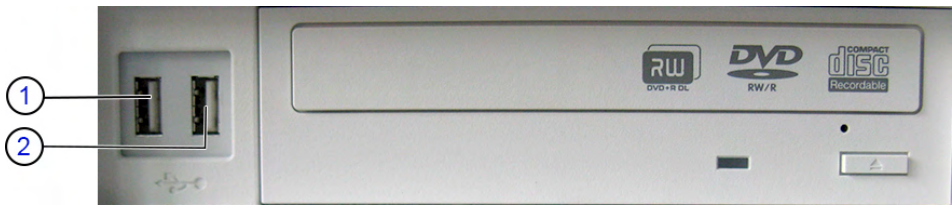
Figure 5-17 External I/O connectors - next to DVD drive
