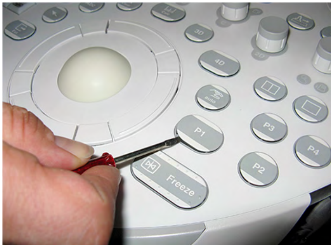
Figure 8-32 push against the circle cap and lift it
