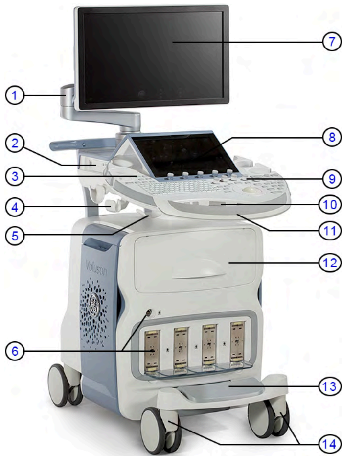
Figure 5-1 Voluson E-Series - Major Components
