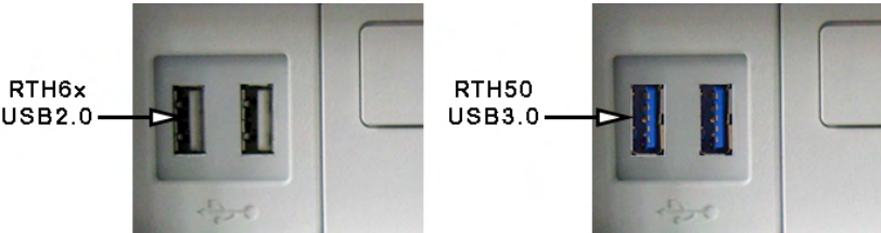
Figure 3-42 RTH6x => "white" USB2.0 ports / RTH50 => "blue" USB3.0 ports
