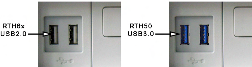
Figure 5-18 RTH6x => "white" USB2.0 ports / RTH50 => "blue" USB3.0 ports
