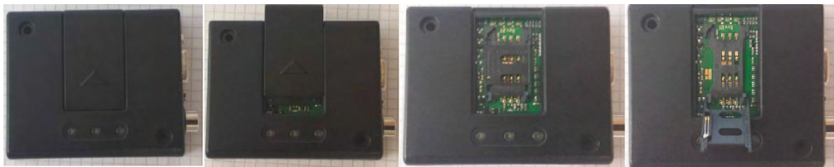
Figure 3-18 open the Cellular Modem cover
