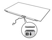
When installing: Make sure that the metal connector is attached firmly.
