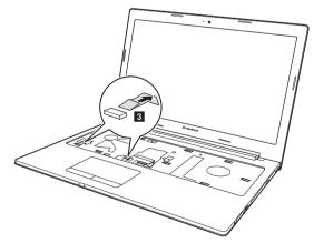
**When installing:** Make sure that the power board connector and touch pad cable are attached firmly.
