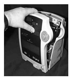
Before the panel can be separated from the case, it is necessary to disconnect the switchboard cable, temperature probe cable and  $SpO_2$  sensor cable if fitted.
