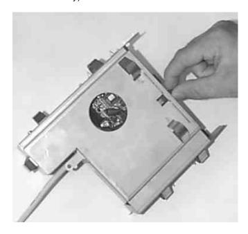
Disconnect pneumatic hose from pump assembly to Main Board secondary pressure transducer on revision 06 units. (Disconnect pressure sensor cable on earlier revisions)
