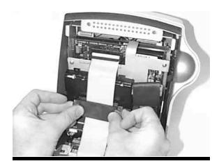
With the ferrite detached, the ribbon cable can be unplugged from socket PL10.
