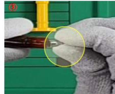
Combine the needle with a syringe to fix it.
