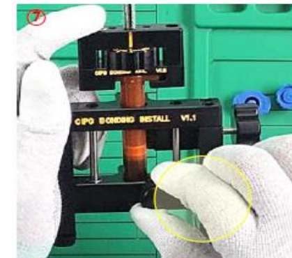
Turn the front knob to fix.
