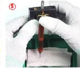
Turn the knob, and squeeze a drop of liquid. And clean the end of a needle.
