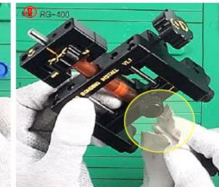
Clean the end of a needle.
