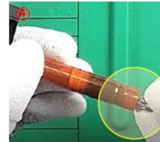
Insert a needle and turn it to fix.
