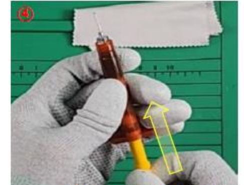
Combine the piston into syringe.
