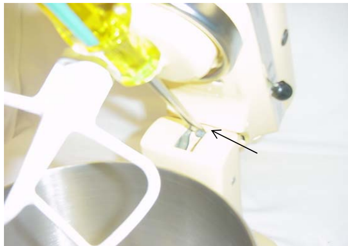
Fig. 83 The beater height adjustment screw used to set the \frac{1}{16} " clearance between the bowl and beater.
