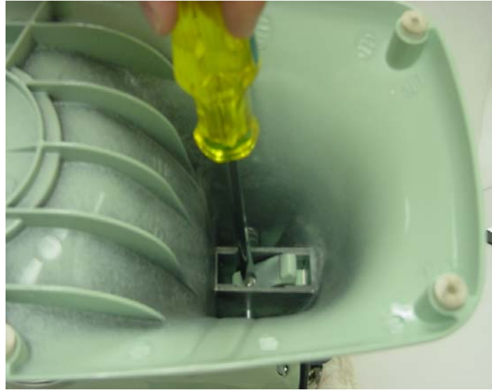
Fig. 3 Loosen the hinge pin setscrew to remove the pedestal from the bottomcover.
