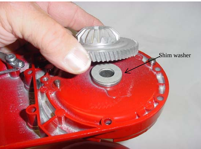
Fig. 55 Bevel center gear being lifted for inspection.
