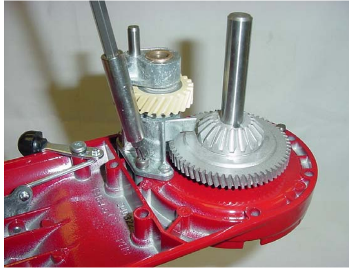
Fig. 52 Worm gear bracket bearing and pin assembly.
