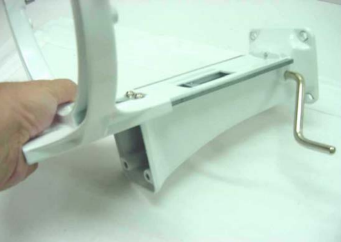
Fig. 88 Slide the bowl support down and off the column to replace the bowl lift assembly.
