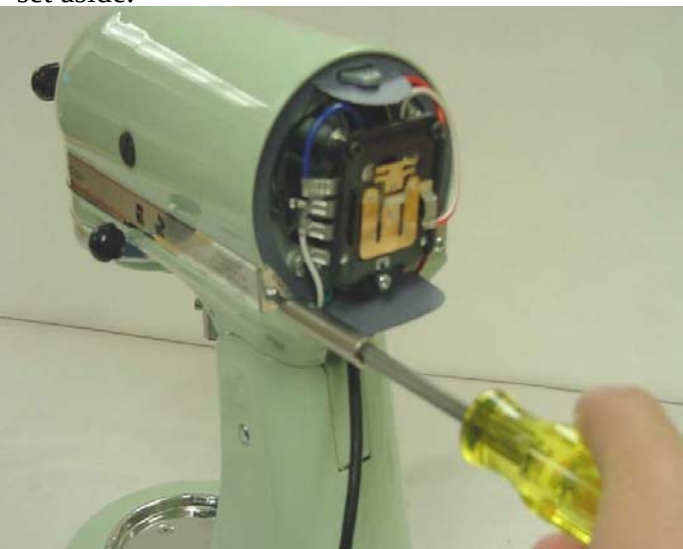
Fig. 2 The trimband can be removed after removing the trimband screws.
