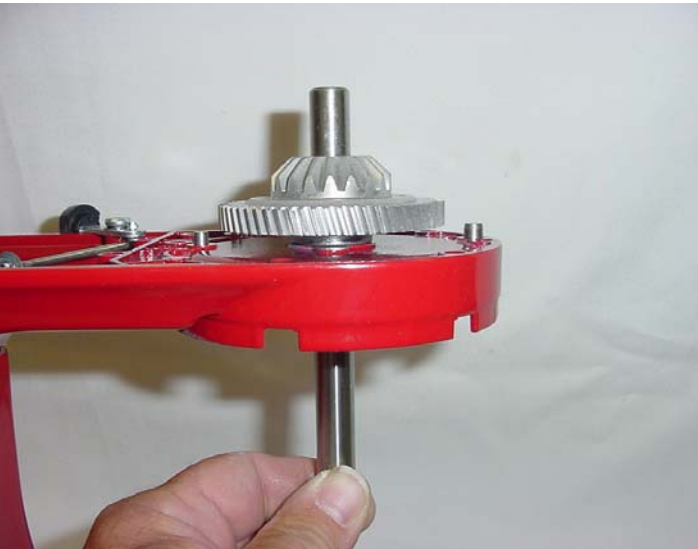
Fig. 54 Removal of vertical shaft from bottom cover.
