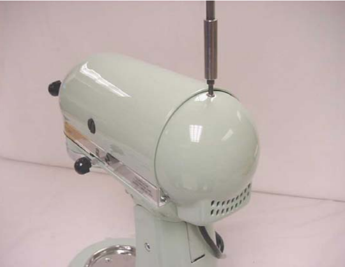
Fig. 1 The end cover is removed by removing the tapered head endcover screw.
