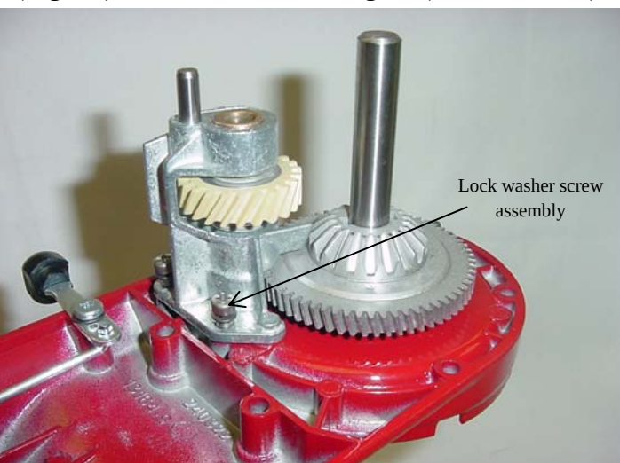
Fig. 59 Secure the three lock washer screw assemblies into the bottom cover.
