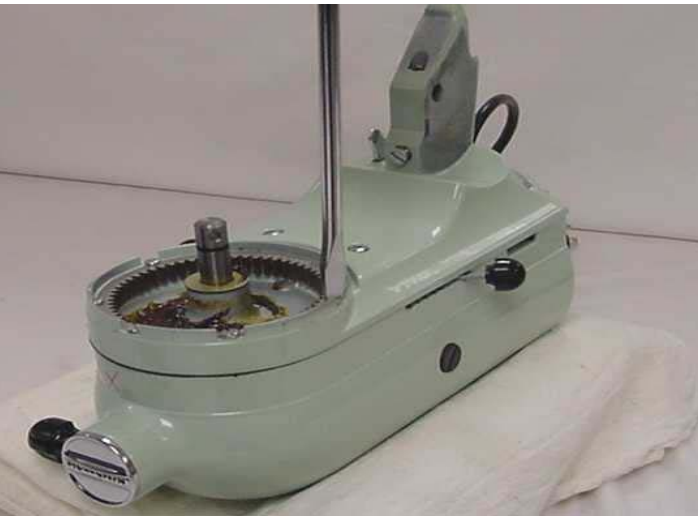
Fig. 10 Removal of the 5 special screws holding the internal gear in the bottom cover.
