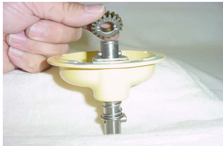
Fig. 65 Lift the pinion off and take out the pin and remove the washer; then pull out the shaft.
