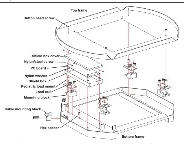
exit points "up". Place the two Philips head screws into the recess in the cable exit support block and locate them through the clearance holes in the scale bottom frame. The "jiffy" clip should be placed on the exposed thread of the left (as viewed from the outside of the scale) screw with the recess in the clip oriented towards the outer wall of the bottom frame. Apply both Keps nuts with the serrated side toward the frame.
