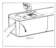
3 Open hinged latch of bobbin case and pull bobbin case out of machine.
