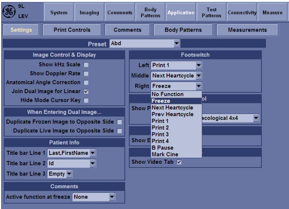
Figure 3-25. Configuring Footswitch Functions
