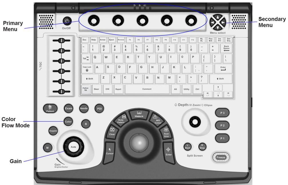
Figure 4-15. Controls available in Color Flow Mode
