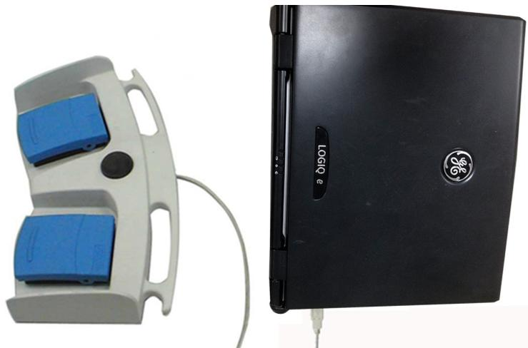
Figure 3-24. Connect Footswitch to the system
