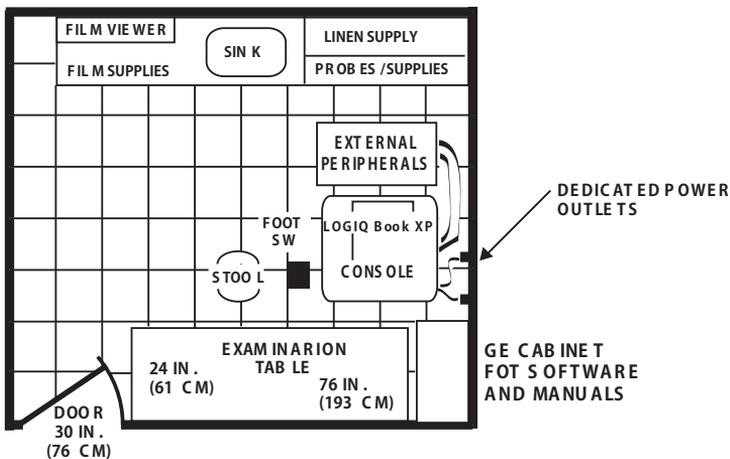
An 8 by 10 foot Minimal Floor Plan
