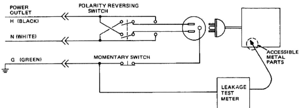
Figure 10-8. Set Up for Chassis Source Leakage Current, IEC 601-1 Clause 19 - Continuous Leakage Currents and Patient, Auxiliary Currents
