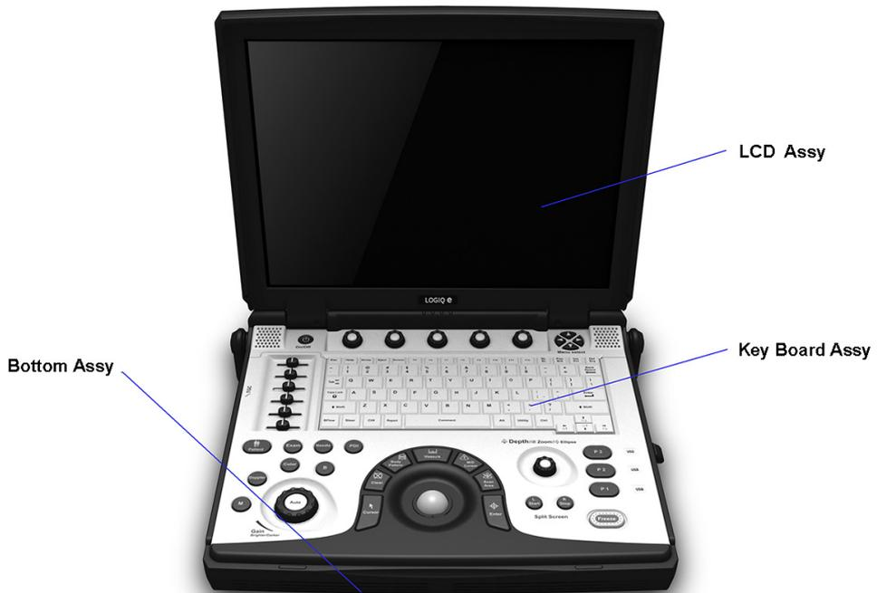
Figure 9-1. Operator Console Assy
