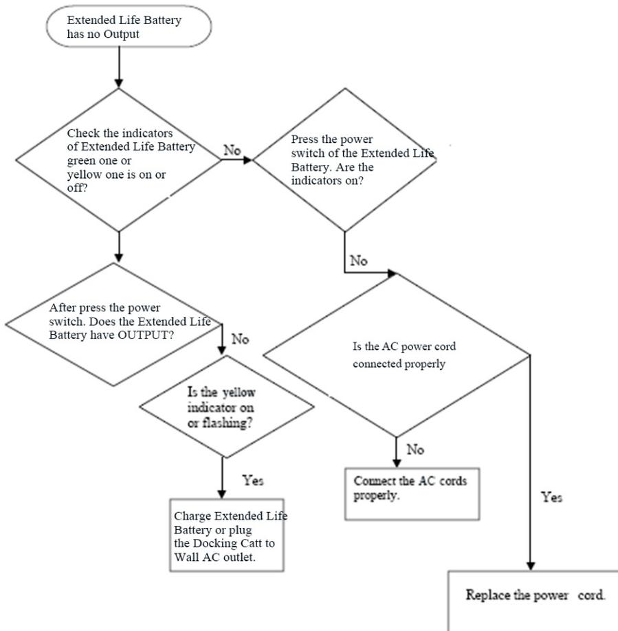
Figure 11-34. Extended Life Battery Has No OUTPUT
