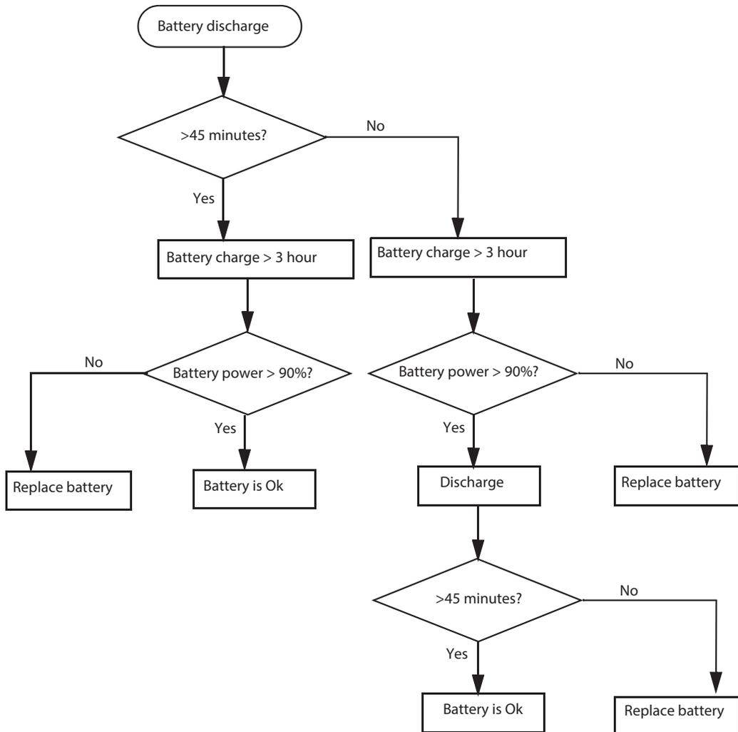
Figure 10-5. Flow chart of Battery Performance Maintenance
