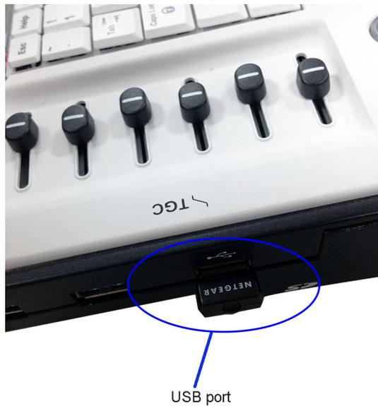
Figure 3-22. Connect Wireless LAN Adapter to the system
