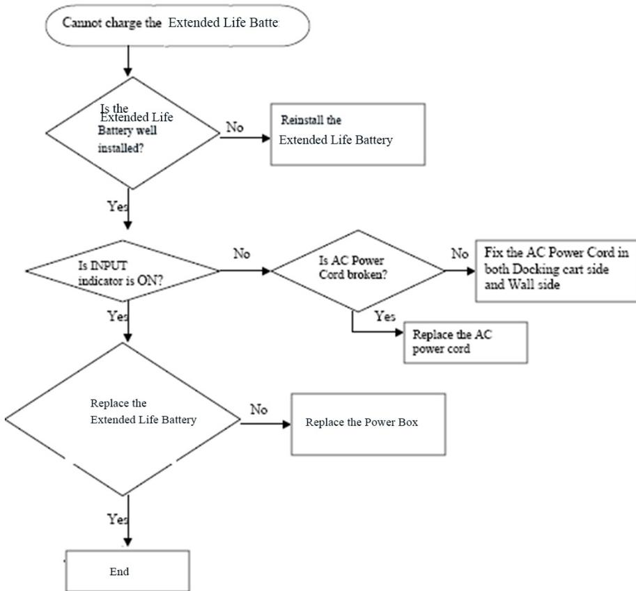
Figure 11-33. Can not Charge the Extended Life Battery
