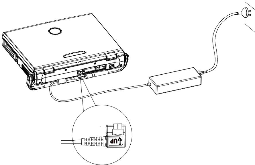
Figure 4-1. Connect AC Adapter
