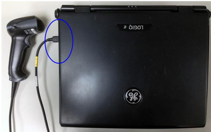
Figure 3-26. Connect Barcode Scanner to the system
