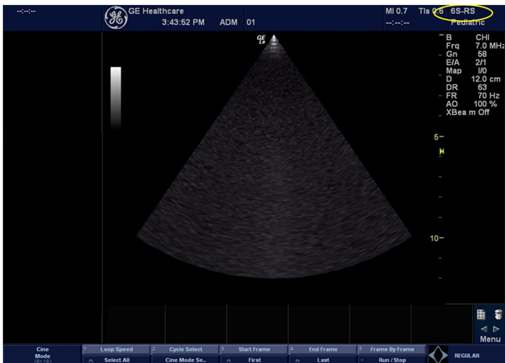
Figure 8-12. Probe identification
