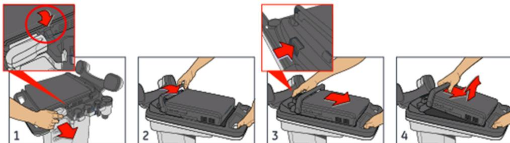
Figure 11-17. Release the System from Cart
