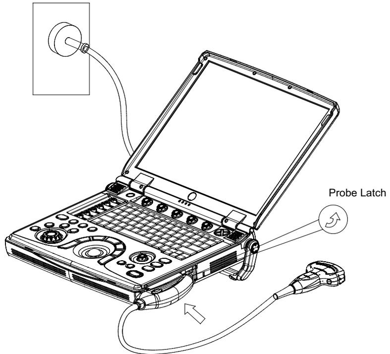
Figure 3-9. Probe connectors
