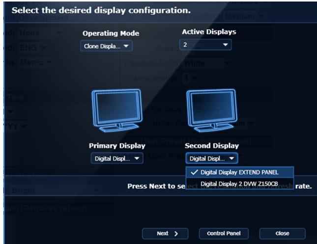
Figure 11-23. Select Digital Display EXTEND PANEL
