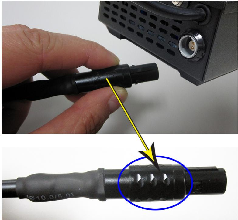
Figure 11-5. Disconnect Power Cable
