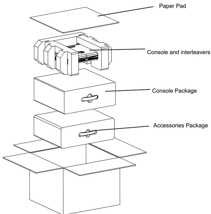
Figure 3-2. Unpacking the equipment
