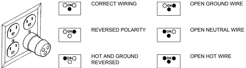
Figure 10-6. Typical alternate outlet tester
