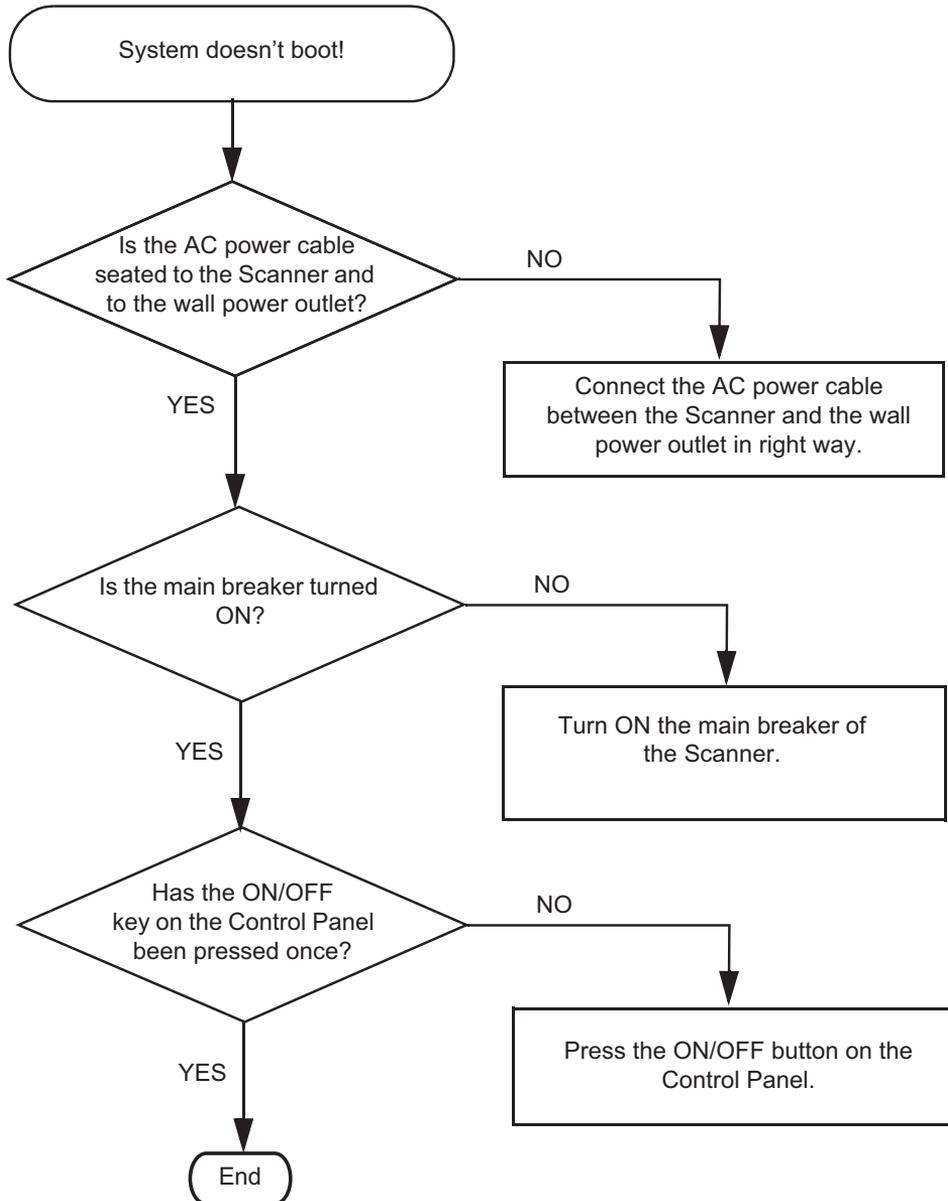
Figure 11-32. System Does Not Boot
