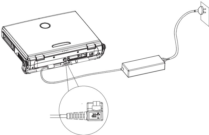
Figure 3-6. Connect AC adapter
