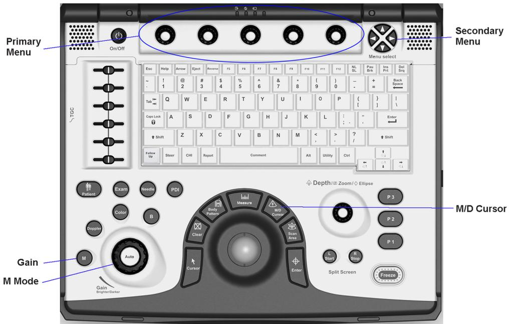
Figure 4-13. Controls available in M Mode
