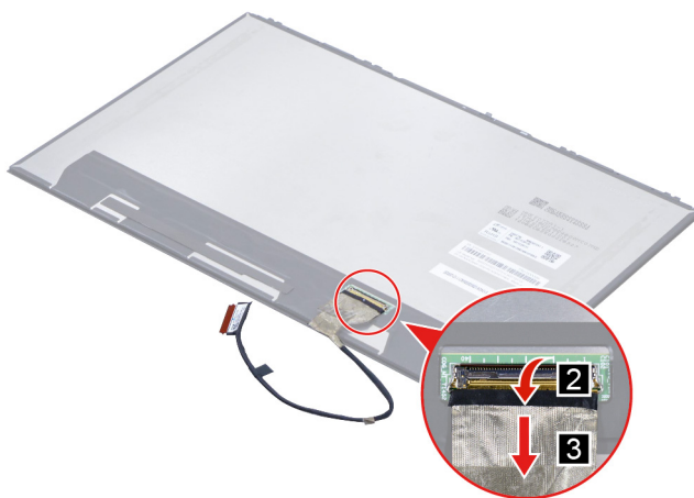
Figure 37. Remove the EDP cable
