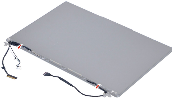
Figure 32. Release the cables from the cable guide
