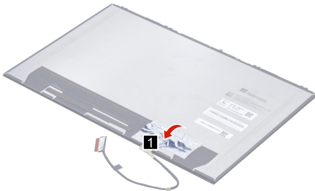
Figure 36. Peel off the tape
