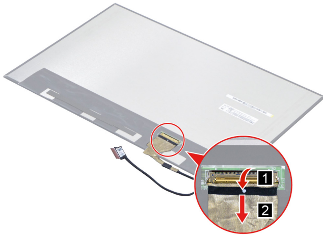
Figure 47. Remove the EDP cable
