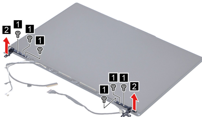
Figure 33. Remove six screws and then remove the hinges
