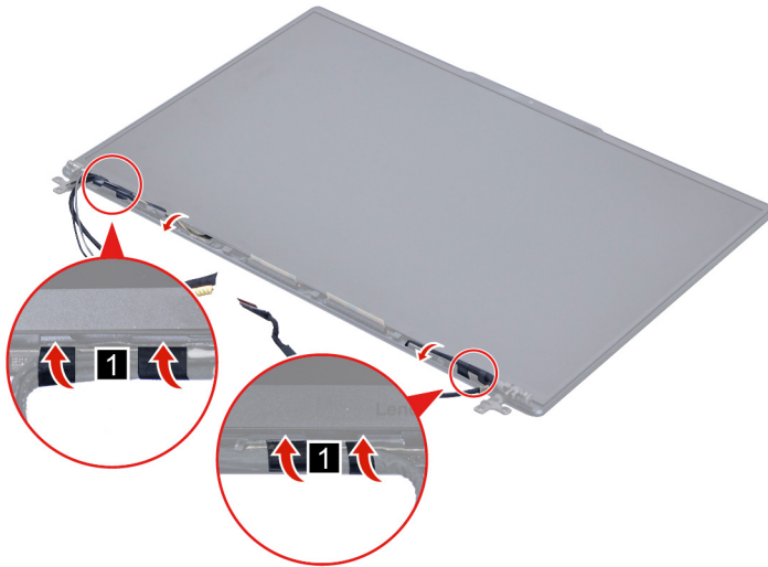
Figure 43. Release the cables from the cable guide
