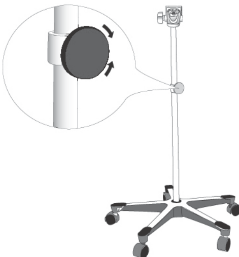
Figure 13. Adjusting the height of the mobile stand.
