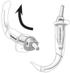
Figure 24. Insert the video baton cable into the Stat.
