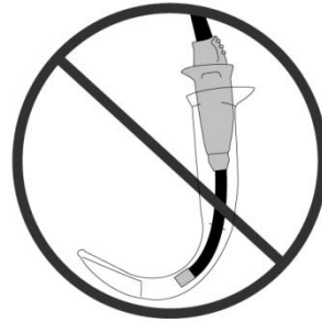
Figure 25. Do not insert the video baton cable into the Stat backward.
