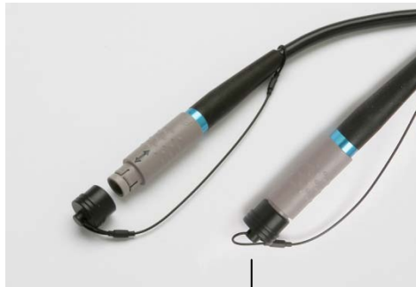
Correct cleaning position – protective cap covering the electronic connector
