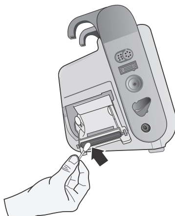
Figure 24-3. Cleaning the Print Head
