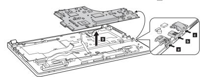
When installing: When attaching the system board to the base cover, adjust the placement of the USB, HDMI, RJ-45 ports as shown in a b c, and make sure that they are attached to the holes on the base cover as shown. Improper placement of those jacks might cause a damage.
