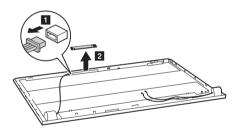
**When installing:** Stick the integrated camera to the top center of the LCD cover and adjust the placement of it to make sure the connector is attached firmly.
