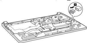
**When installing:** Make sure that the fan connector is attached firmly to the system board.
