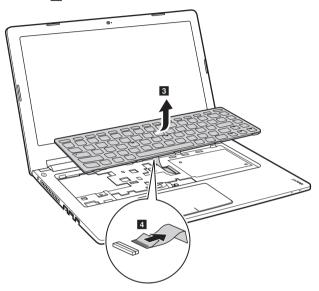
**When installing:** Make sure that the FPC connector is attached firmly.
