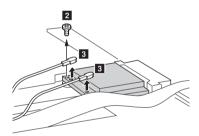
In step **2**, unplug the jacks by using the removal tool antenna RF connector (P/N: 08K7159), or pick up the connectors with your fingers and gently unplug them in the direction shown by arrows.
