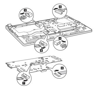
When installing: Make sure that all the connectors are attached firmly.
