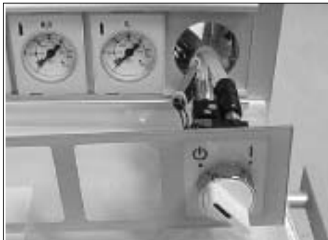
System Switch Telemechanique
