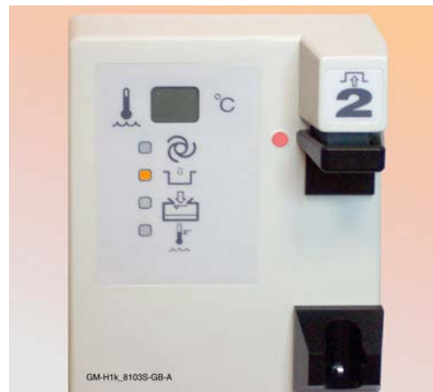
Figure 1 - 8: Alarm - Disposable not correctly fitted, possibility of leak!
