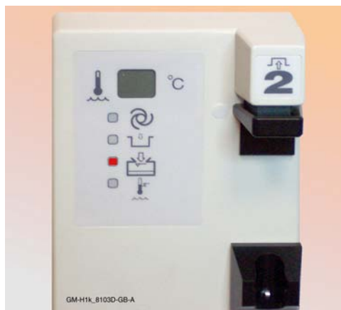
Figure 1 - 6: Alarm - Recirculating Solution Level Low
