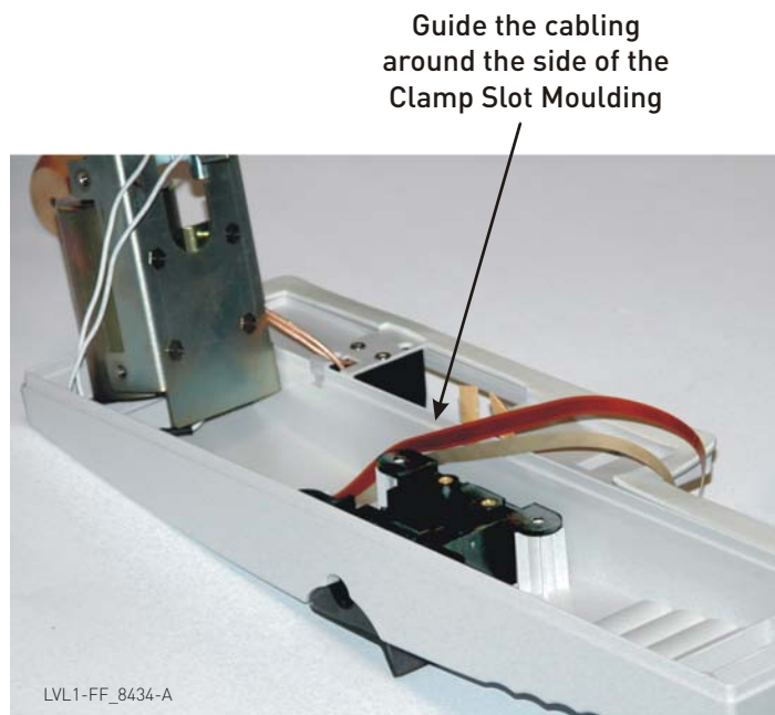
Figure 4 - 39: Ribbon Routing
