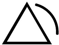
Figure 3 - 17: The "Alarm Test" button has this symbol
