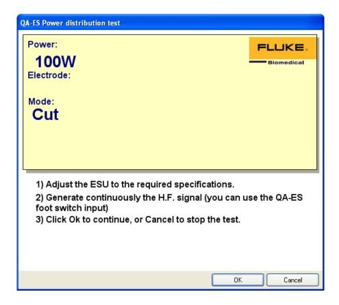
If the setup is identical between two measurements, or when running an RECM Alarm test, this prompt will not be displayed.
