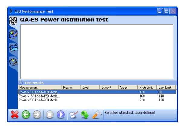
Prior to each measurement within a test the software will display a prompt for the user to set the power, set the mode and set up the next electrode as desired by the particular test.
