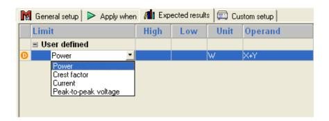
The exception is the power value. The user defined power value in the **test details** box against each measurement is the desired value, naturally. The limits define the acceptable range around this desired power value.
