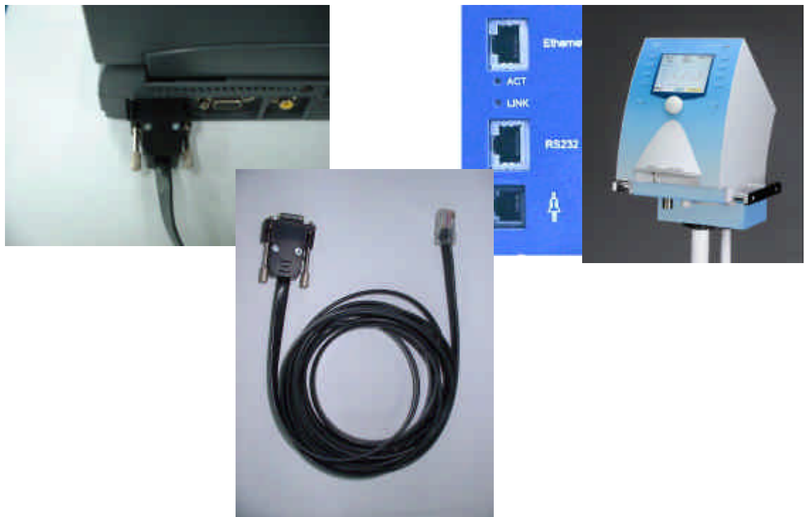
Figure 1, Download Cable Connection
