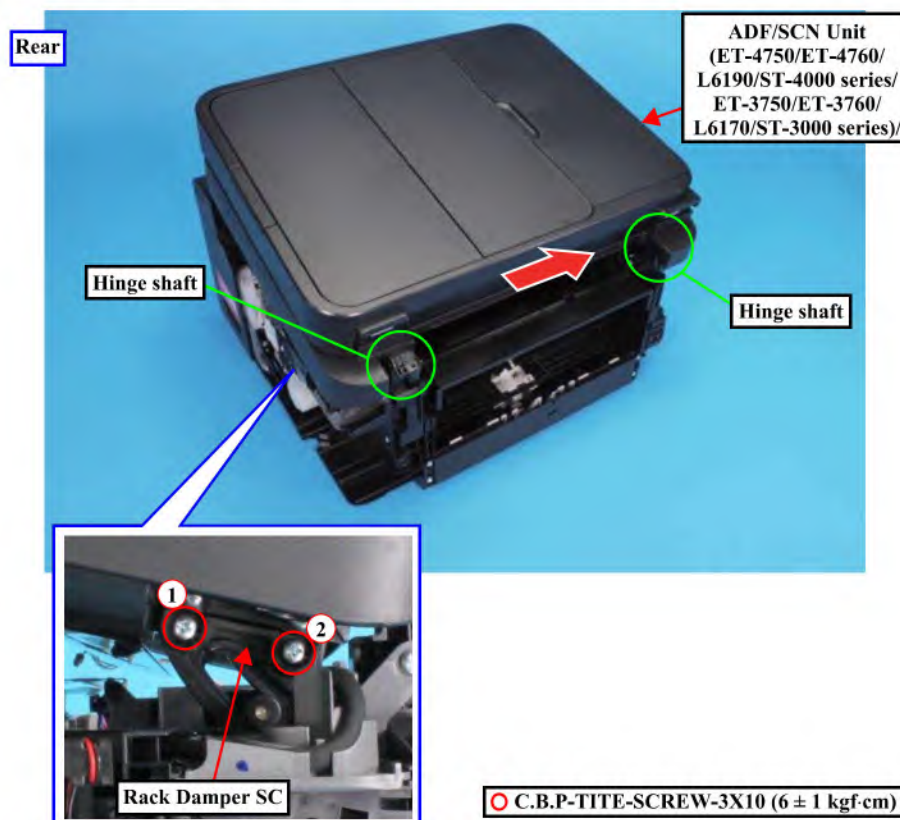
Figure 3-33. Removing the ADF/SCN Unit or the SCN Unit
