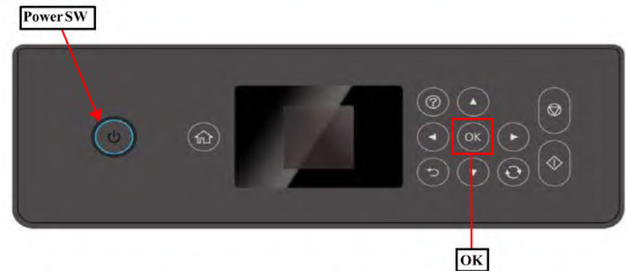
Figure 2-6. Service Support Mode startup and operating procedures
