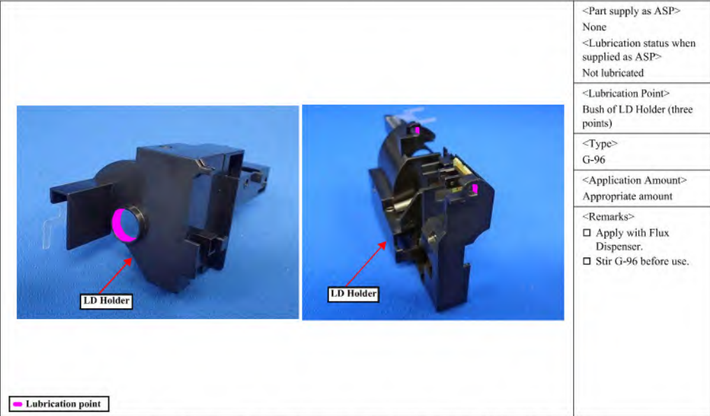
Figure 5-12. Lubricating LD Holder (ET-2750/ET-2760/L4160/ST-2000 series/ET-2700/L4150 series only)
