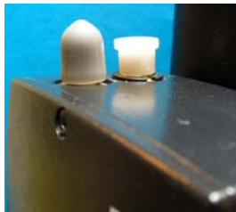
Pic. 54a connector on top of scanner box with protective caps
