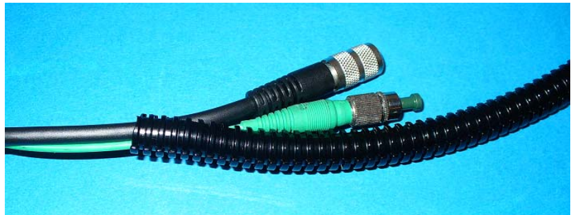
Pic. 44 Fit in glass fiber and scanner cable into the slit of the tube
