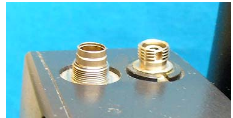
Pic. 54b Left: electrical socket, right: fiber socket
