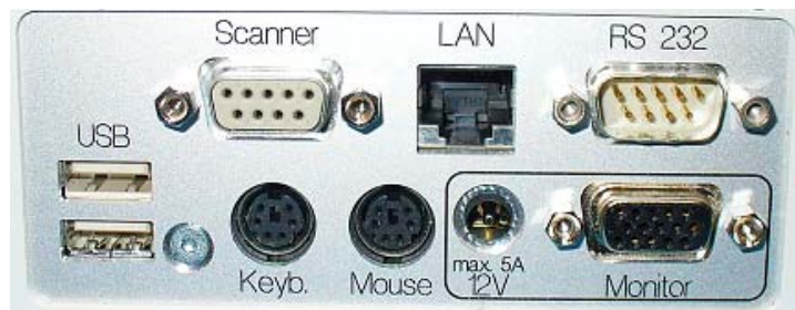
Pic. 60 Connectors of the OCT-box
