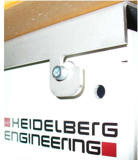
Pic. 38d OCT-Box with fastened screw
