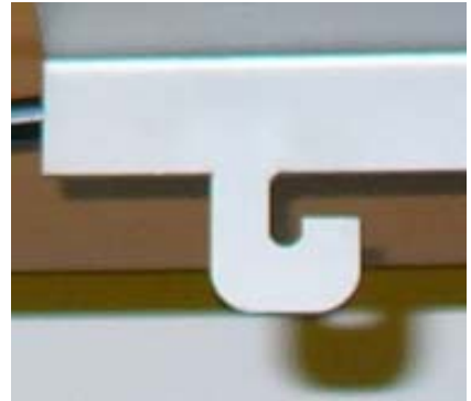
Pic. 38b Hook for hanging the OCT-box beneath the table
