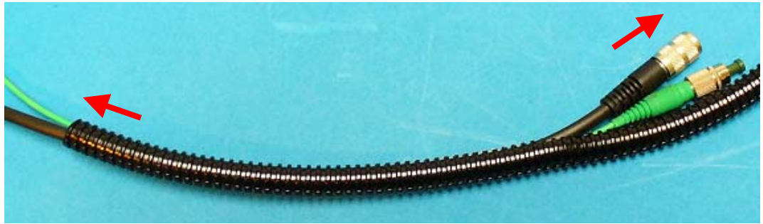
Pic. 45 Glass fiber and scanner cable are sliding into the tube
