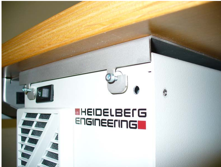
Pic. 38c OCT-Box hanging beneath the table
