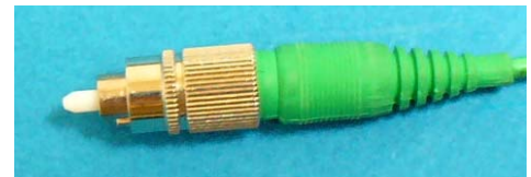
Pic. 55b fiber plug without protective cap
