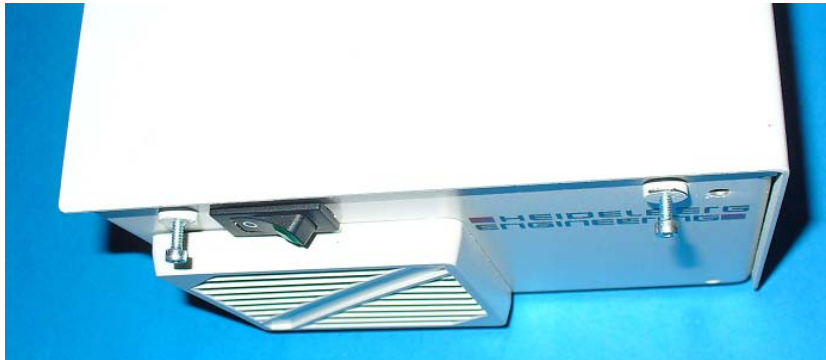
Pic. 38a OCT-Box with premounted screws
