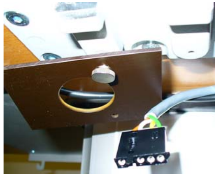
Pic. 22a Protective cover of headrest's electrical plug
