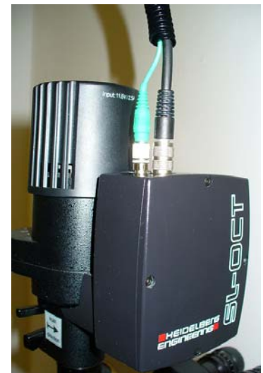
Pic. 57b Glass fiber well guided
