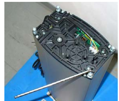
Pic. 8 Premounted screws for assembly of the foot
