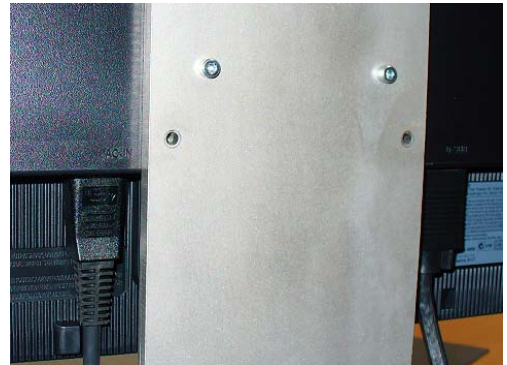
Pic. 61b Monitor with ac power supply (left) and VGA connection (right)
