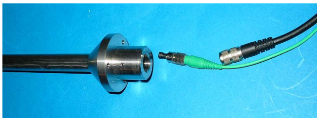
Pic. 41b Fiber and electrical connector
