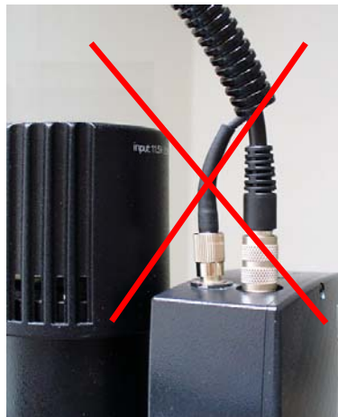
Pic. 57a buckled fiber
