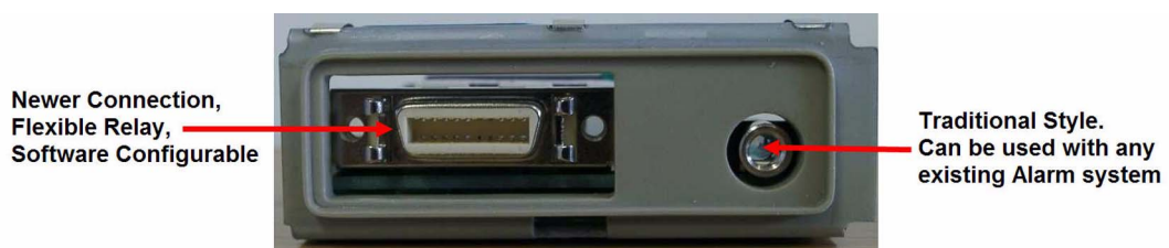
Flexible Nurse Call Relay Connections at Monitor
