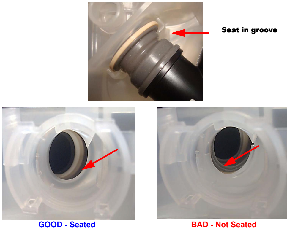
FIGURE 7-25: BLOWER OUTLET SEAL ALIGNMENT
