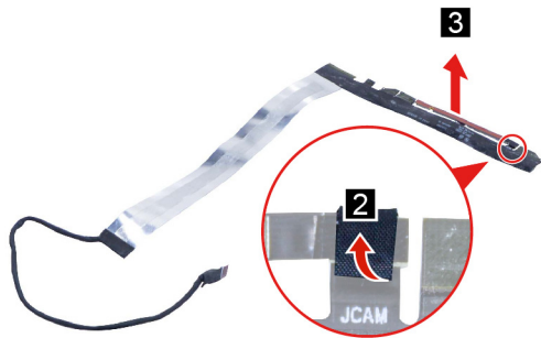
Figure 36. Detach the camera cable connectors and then remove the camera cable
