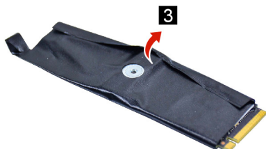
Figure 7. Remove the SSD mylar
