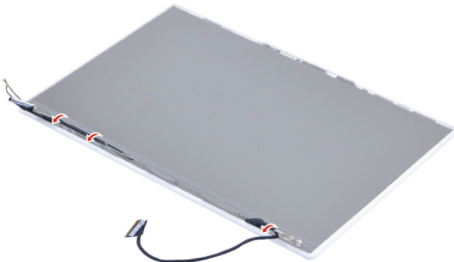
Figure 27. Release the EDP cable and camera cable from the cable guide
