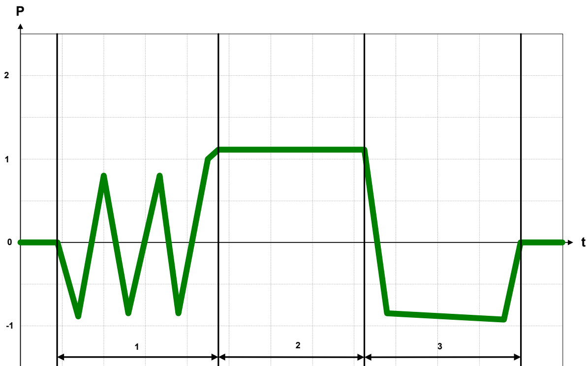
Figure 7-5: Cycle Graph - 121°C Rubber cycle
