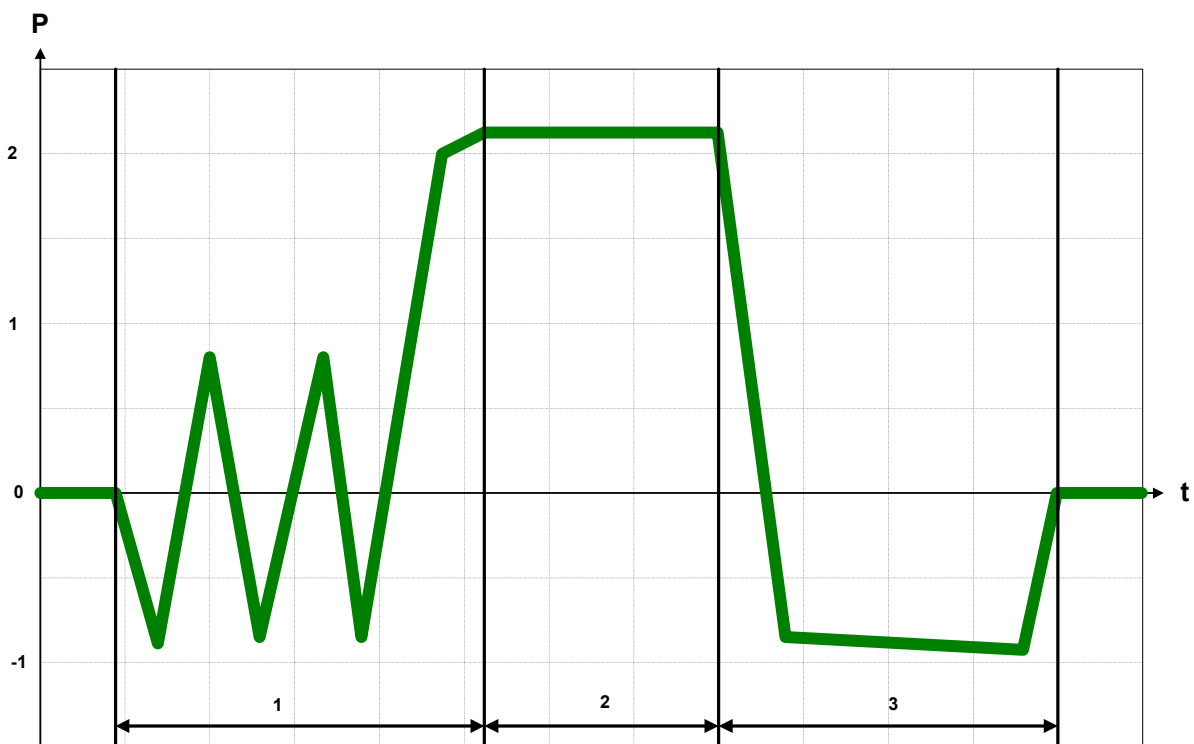
Figure 7-4: Cycle Graph - 134°C Porous load cycle
