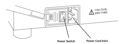
**To turn the instrument ON**, switch the **Power Switch (O/I)**, adjacent to the power connector, to the ON **(I) position**. The instrument will perform internal self-diagnostic checks and after approximately 15 seconds, two double beeps will sound and the **FDT MAIN MENU** will appear on the Operator LCD Display. Refer to the troubleshooting section of this manual if the **FDT MAIN MENU** does not appear.
