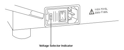
To change the Fuse Carrier/Voltage Selector to the proper operating voltage be sure the Power Cord is NOT connected and use a flat screwdriver to pry open the Fuse Drawer Cover. Remove the
