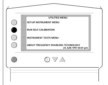
**Note**: Be sure to **cover** the **Patient Eyepiece** with the Calibration Cap shipped with each unit. If the Calibration Cap is not available, substitute something that will temporarily block light from entering the Patient Eyepiece or perform the calibration in a completely darkened room (black cloth over Patient Visor, etc.). The Operator LCD Display will indicate if there is too much ambient light to complete the calibration.
