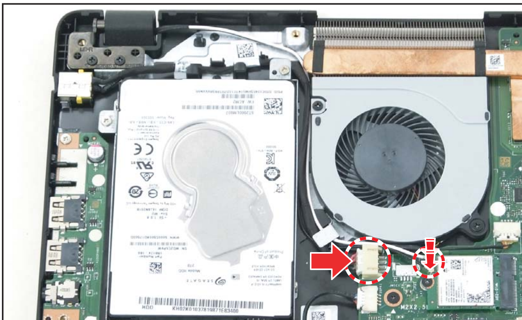
Figure 5-120. Connecting the Cables
