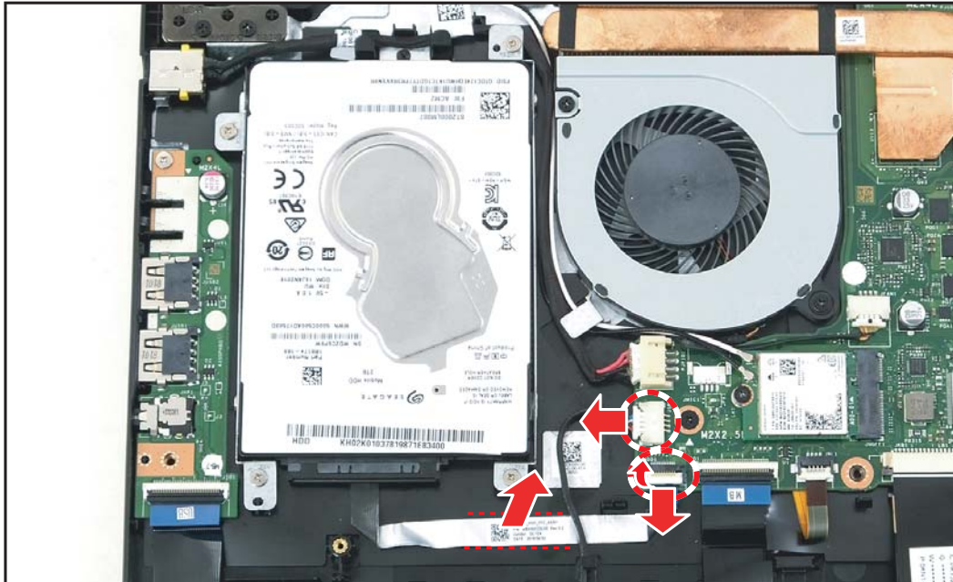
Figure 5-20. Disconnecting the Cables
