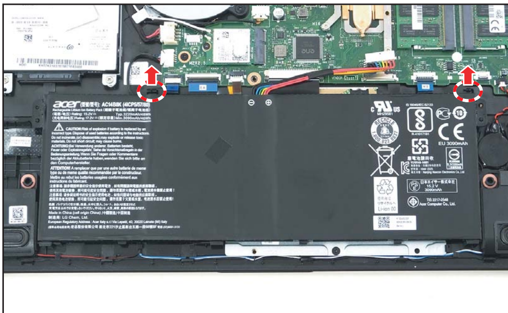
Figure 5-14. Releasing the Upper Tabs of the Battery
