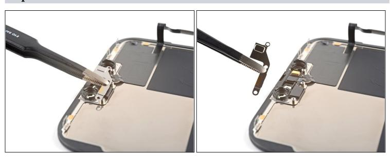
• Use <u>tweezers</u>, or your fingers, to remove the front sensor assembly bracket.
