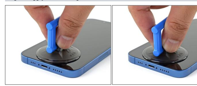
• If you're using a single suction handle, apply it to the bottom edge of the phone, while avoiding the very edge of the glass.
