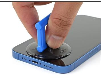
• If you're using a single suction handle, apply it to the bottom edge of the phone, while avoiding the very edge of the glass.
