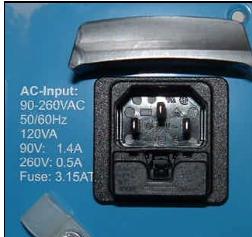
Fig 3-26, Power Entrance Module
