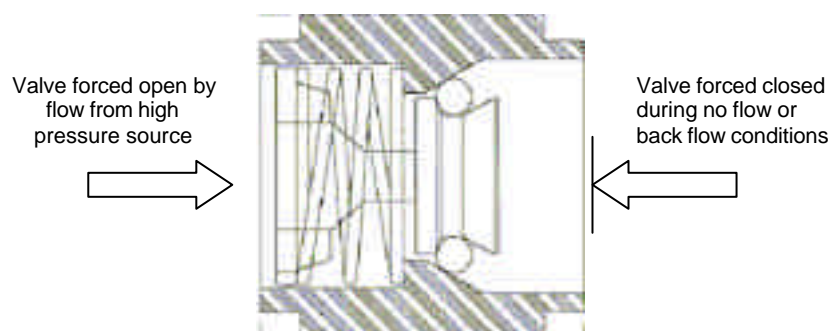
Fig 3-5, Section Through Check Valve
