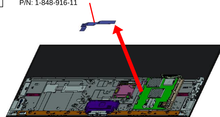
FLEXIBLE FLAT CABLE 51P (XBS) P/N: 1-848-916-11
